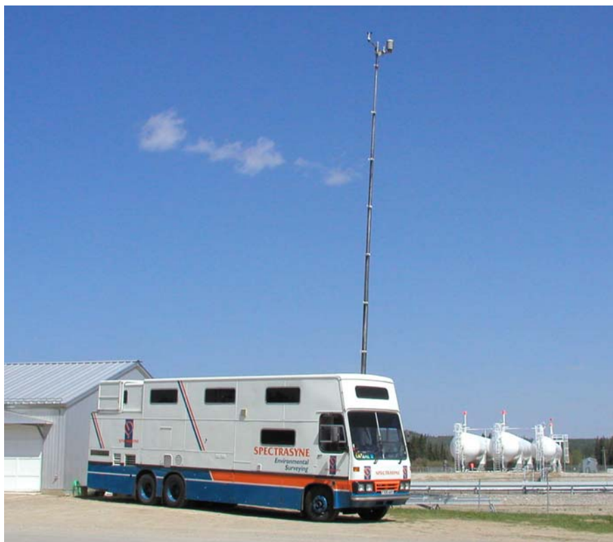
Figure 1: Spectrasyne DIAL Unit Measuring Fugitive Emissions at a Gas Plant in Alberta
