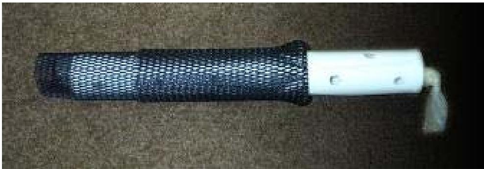
**Figure 2-5. Regenerated Cellulose Dialysis Membrane Diffusion Sampler With Perforated PVC Pipe Support Inside the Membrane**
