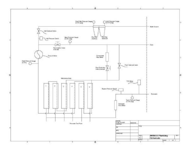
Figure 2-2: Watts Premier M-15,000 RO Treatment System process flow diagram and sample locations.
