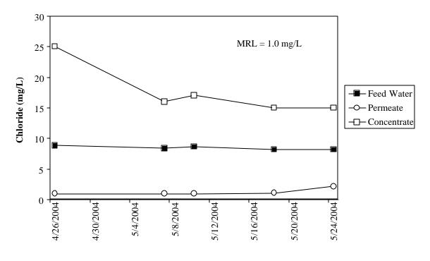
Verification Testing Figure 4-13: Temporal plot of chloride.
