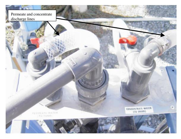
**Photograph 1: Permeate and Concentrate Discharge Lines**
