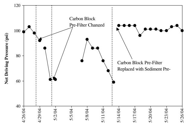
Figure 4-7: Temporal profile of net driving pressure.
