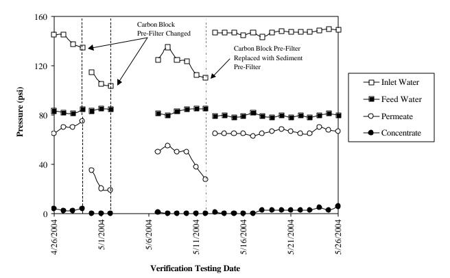
Figure 4-2: Average daily feed water, inlet, back pressure, and tank pressures.
