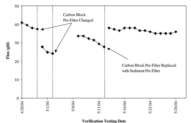
Figure 4-4 Temporal plot of flux verses time.
