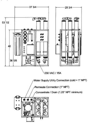
Figure 2-1: Watts Premier M-Series M-15,000 RO Treatment System.
