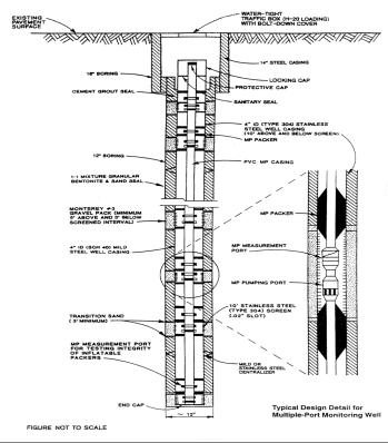
Westbay System multi-port monitoring systems are complex and require trained technicians to install. Monitoring wells must be designed specifically to conform with the Westbay System requirements. Field quality control procedures enable verification of the quality of the well installation and operation of the testing and sampling equipment.
