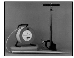
Solinst also manufactures a Triple Tube Sampler that uses a narrow-diameter pump and packer assembly to seal off a discrete
