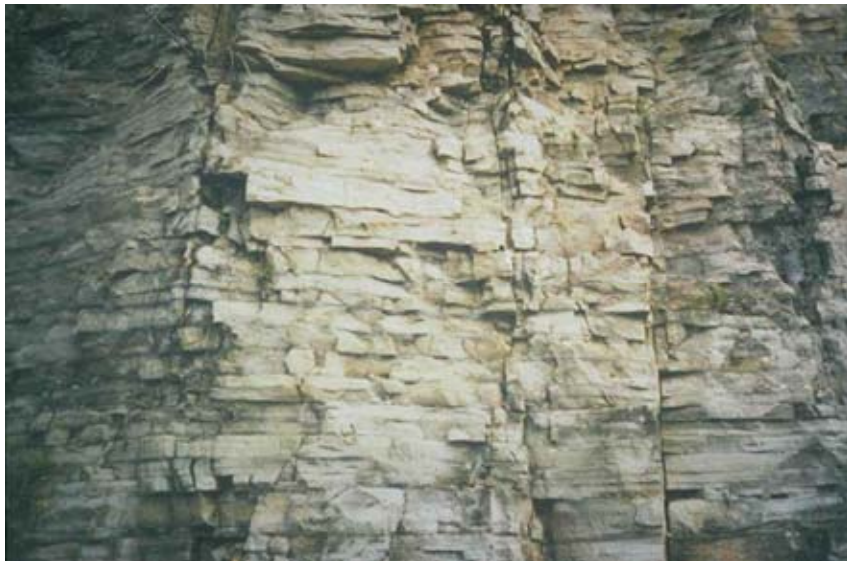
Figure 9 - Bedding planes, joints, and vertical fractures in carbonate rock, Ontario, Canada (Photo Courtesy of Dr. Beth Parker University of Guelph).
