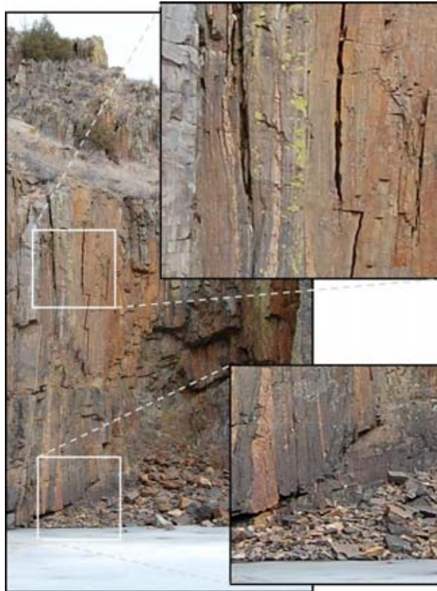
Figure 8 - Fractured crystalline rock, an example of Type IV media (Cache La Poudre River, Colorado, Photo provided by Tom Sale) .
