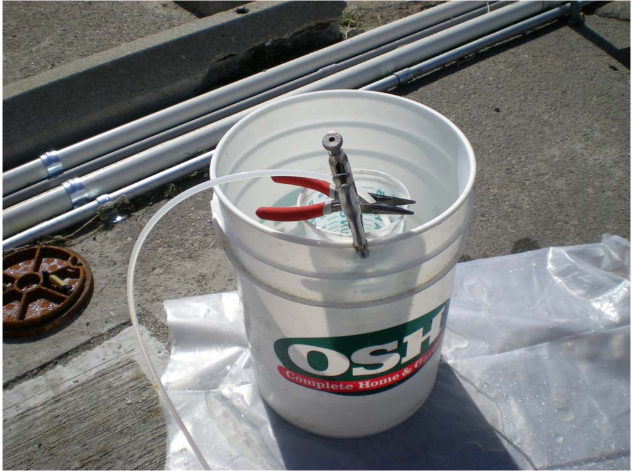
Picture 16. Purging groundwater into bucket.
