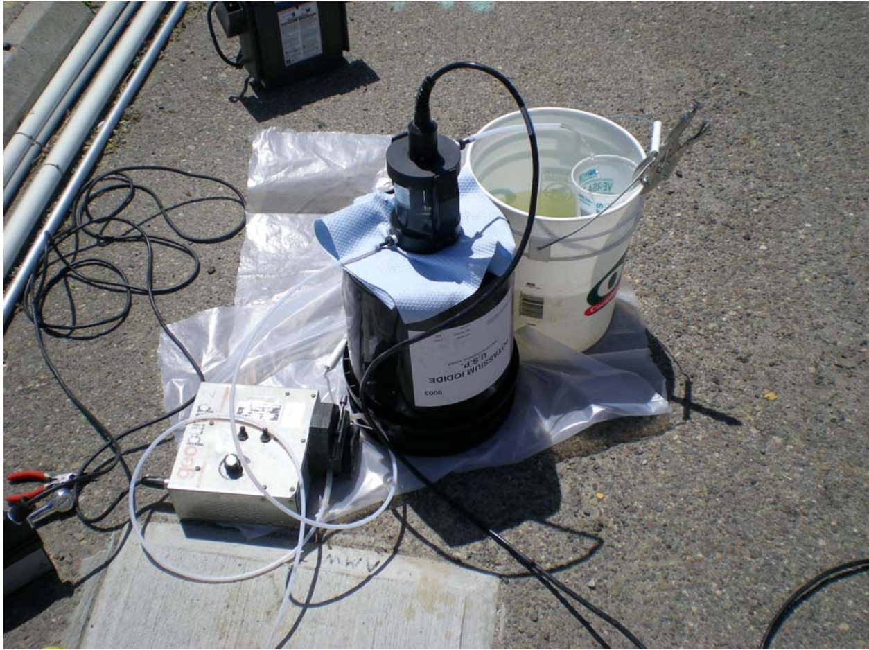
Picture 15. Groundwater purge setup with YSI.
