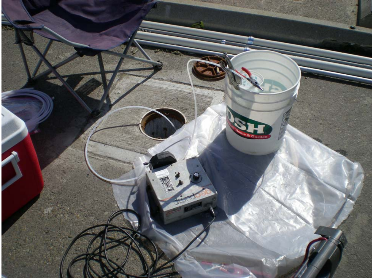
Picture 10. Peristaltic pump sampling setup.
