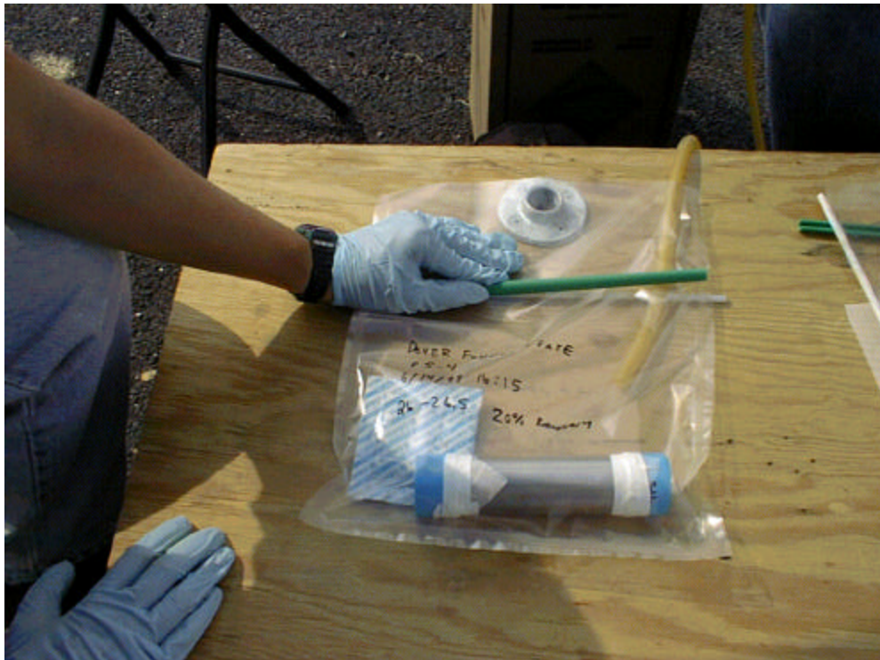
Figure 8-12. Tedlar™ Bags Flushed with Nitrogen Gas Before Sealing
