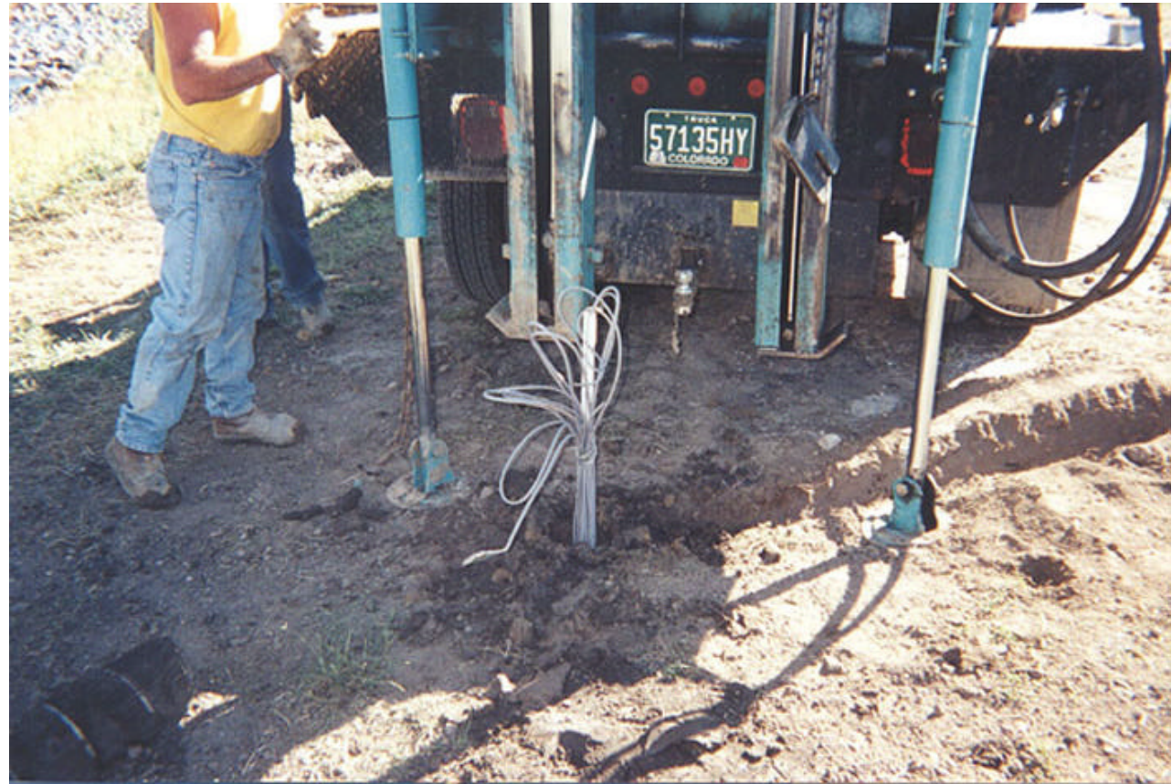
Figure 8-5. Pictures of (a) an In Situ Groundwater Velocity Sensor and (b) Its Installation
