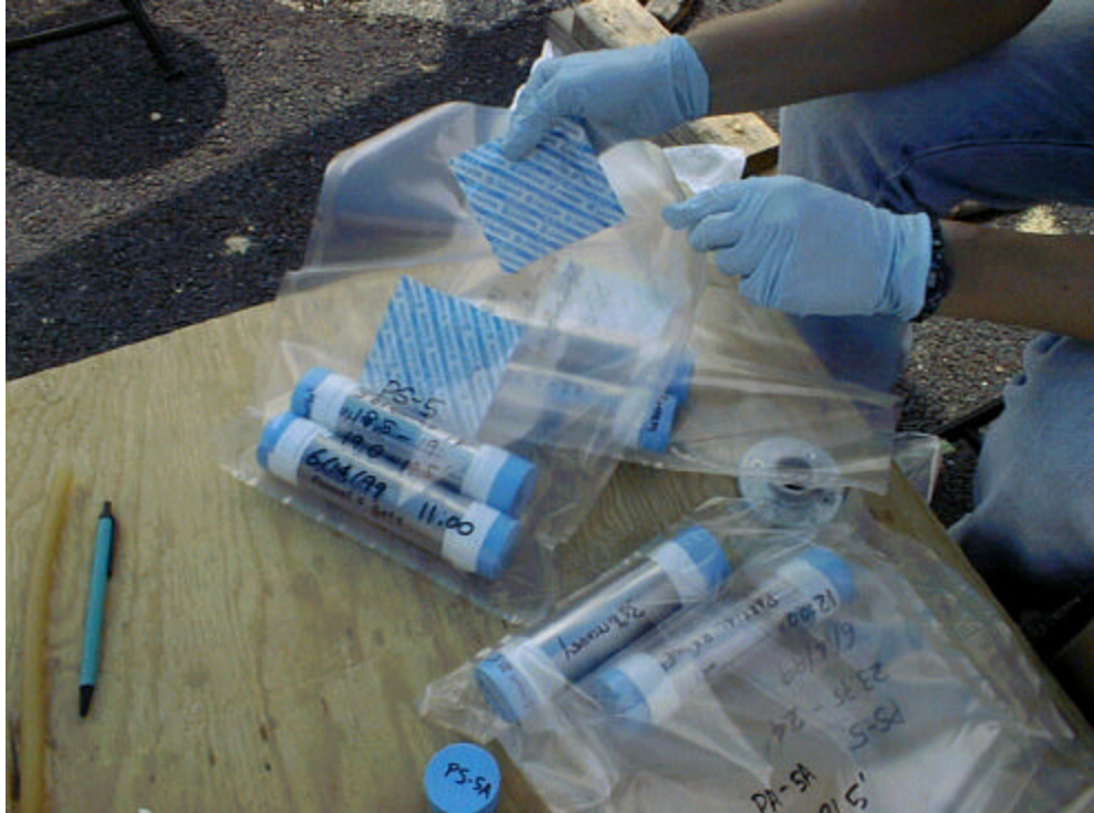
Figure 8-11. Photograph of Core Sleeves Being Placed into Tedlar™ Bags that Contain Packets of Oxygen Scavenging Material
