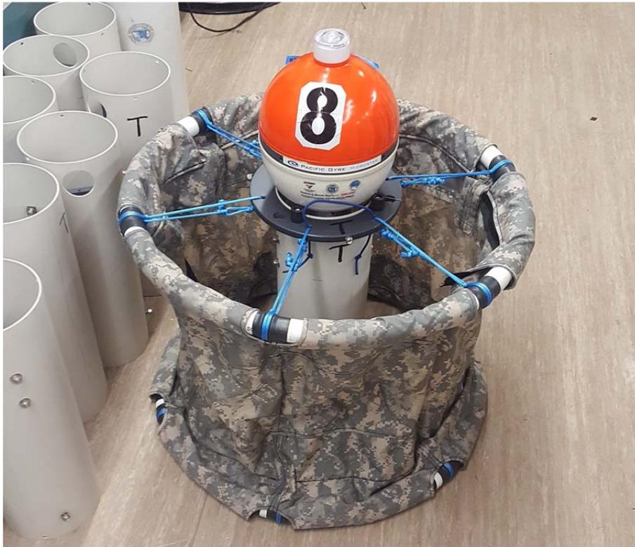
**Figure 48. DPS system with the drogue size reduced for shallow water operations during the Waiiau event.**
