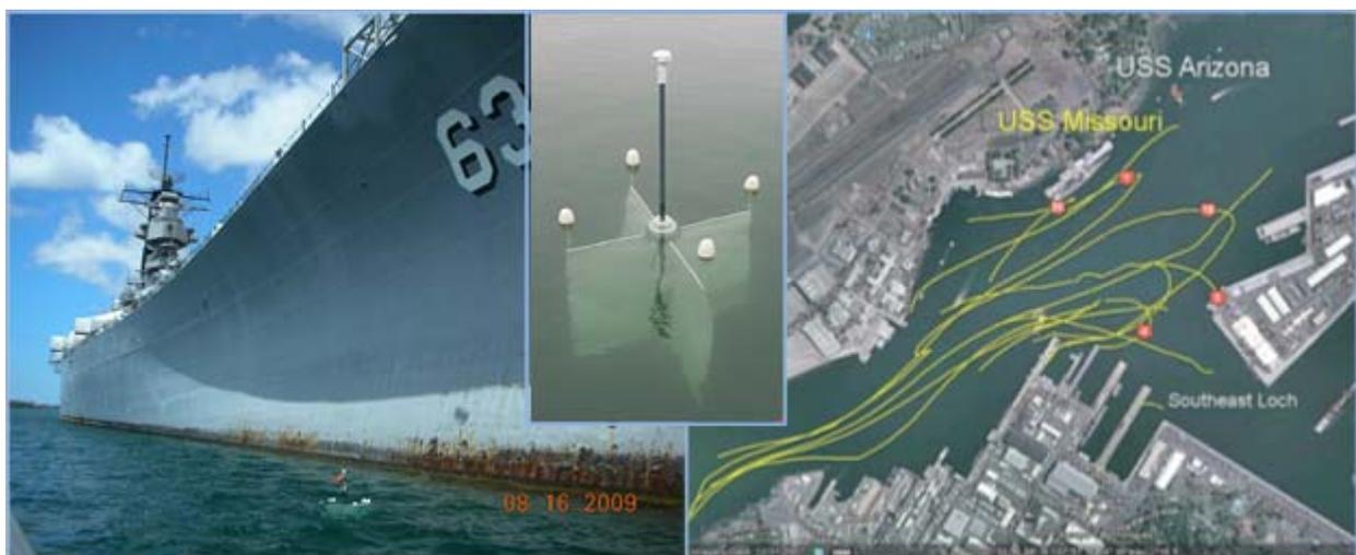
**Figure 2. Davis/CODE drifter (center) shown deployed in Pearl Harbor near the USS Missouri (left) and the resulting trajectories (right).**
