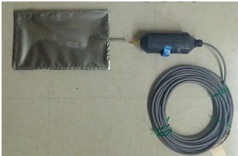
**Figure 4. Load cell scour sensor showing pressure plate and standard dual pressure.**
