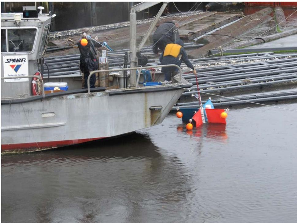
**Figure 35. DrEx drifter being released into the flow from Paleta Creek during the Jan 5-6, 2016 event.**
