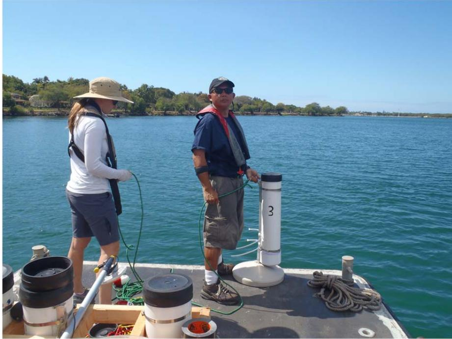
**Figure 45. Preparing to install a sediment trap at the Oscar Pier site.**
