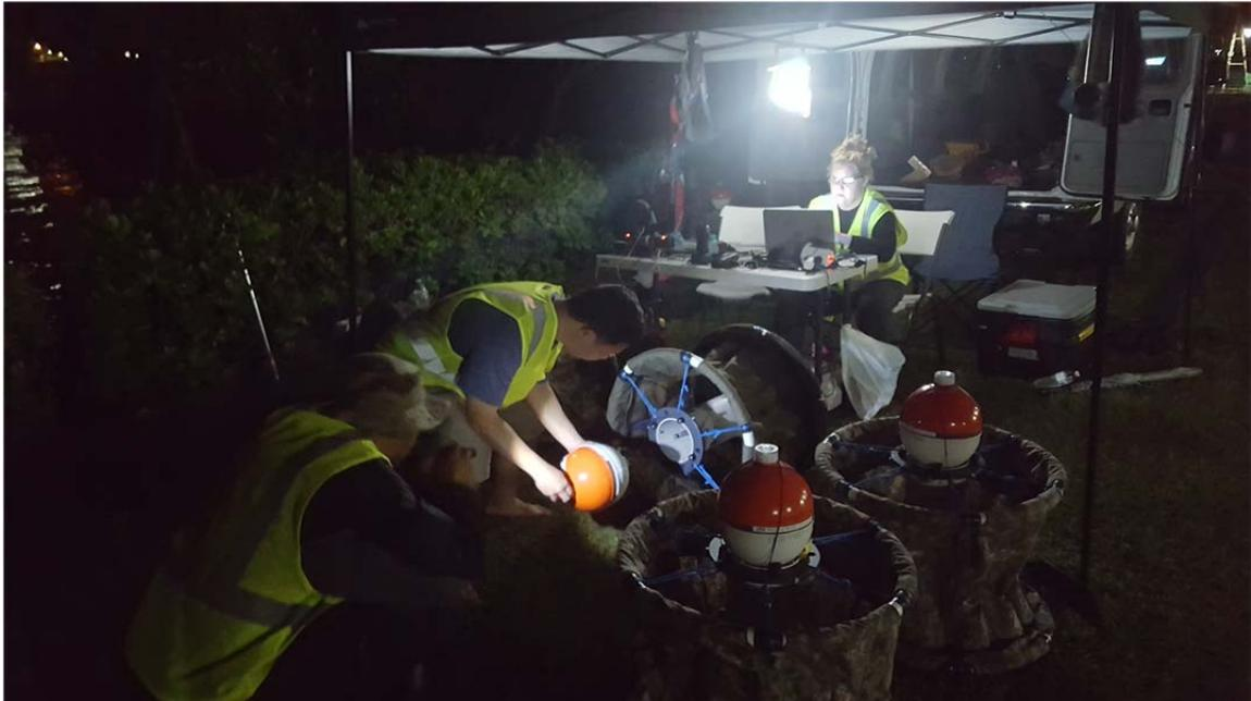
Figure 49. Testing the DPS winch and preparing the unit for deployment during night operations at the Waiiau site.
