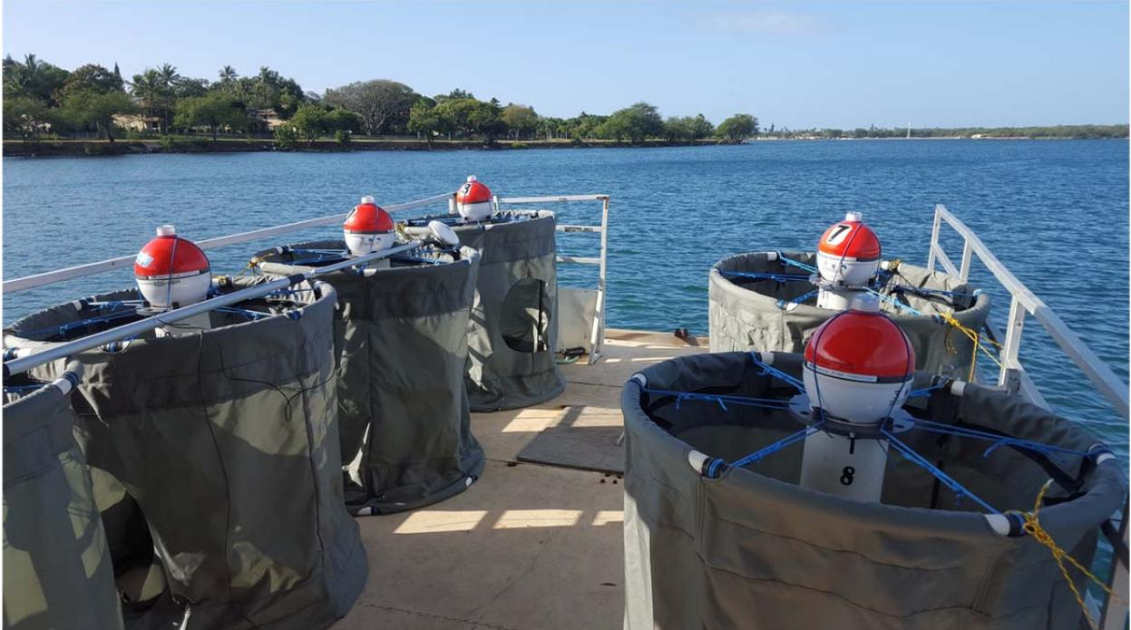
**Figure 39.** The DPS units prepared for deployment onboard the survey boat in Pearl Harbor.
