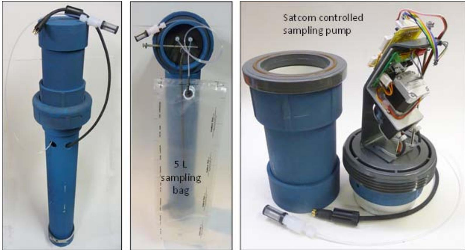
**Figure 7. The Programmable Automatic Water Sampler (PAWS) unit.**
