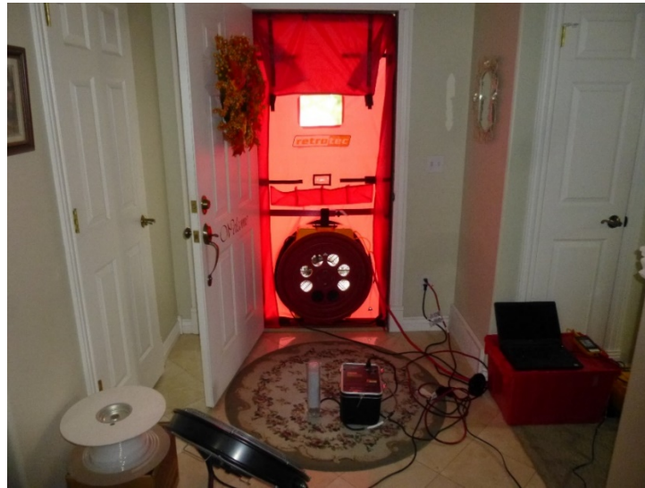
Figure 3. Blower door installation and the use of floor fans to facilitate air mixing near the blower intake sampling area.
