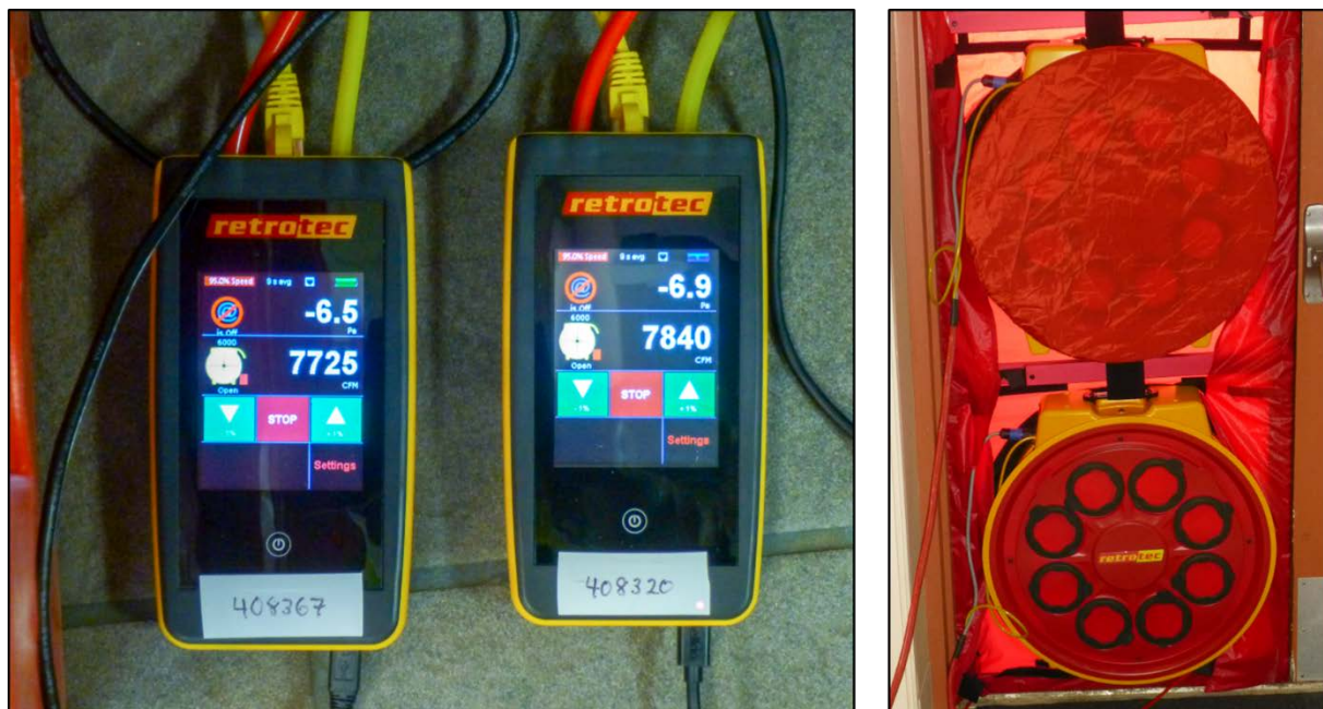
Figure 2. Retrotec DM32 with display (left) and blower door with a 2-blower door cloth and blowers (right).
