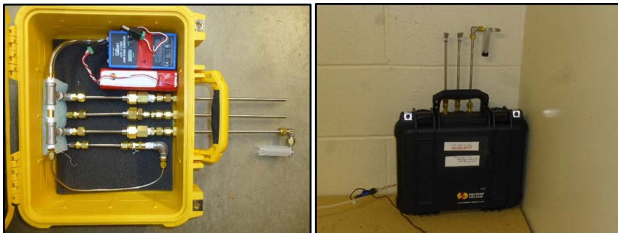
Figure 6. Active TD tube and Passive sampler deployment with passive sampler, TD tube active samplers in triplicate with a single tube for breakthrough assessment, pump, and timer.
