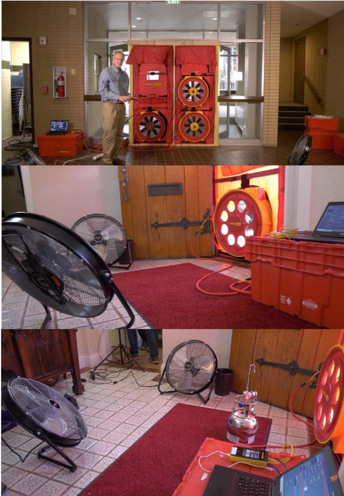
Figure 4. Photos from an industrial multi-blower and residential single blower door CPM test deployment.
