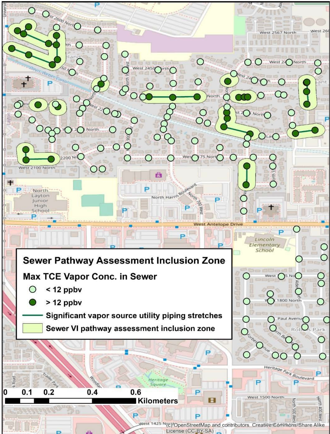
Figure 6.15. Significant Vapor Source Sewer Manholes and Utility Piping Stretches and Corresponding Sewer VI Pathway Assessment Inclusion Zones.
