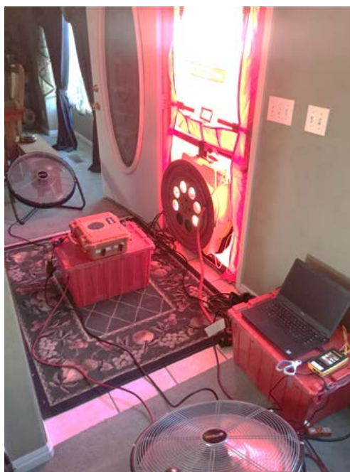
Figure 3. Blower door installation and the use of floor fans to facilitate air mixing near the blower intake sampling area.
