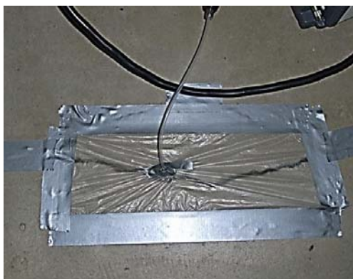
Figure 4: Testing a Sealed Crack in a Concrete Floor
