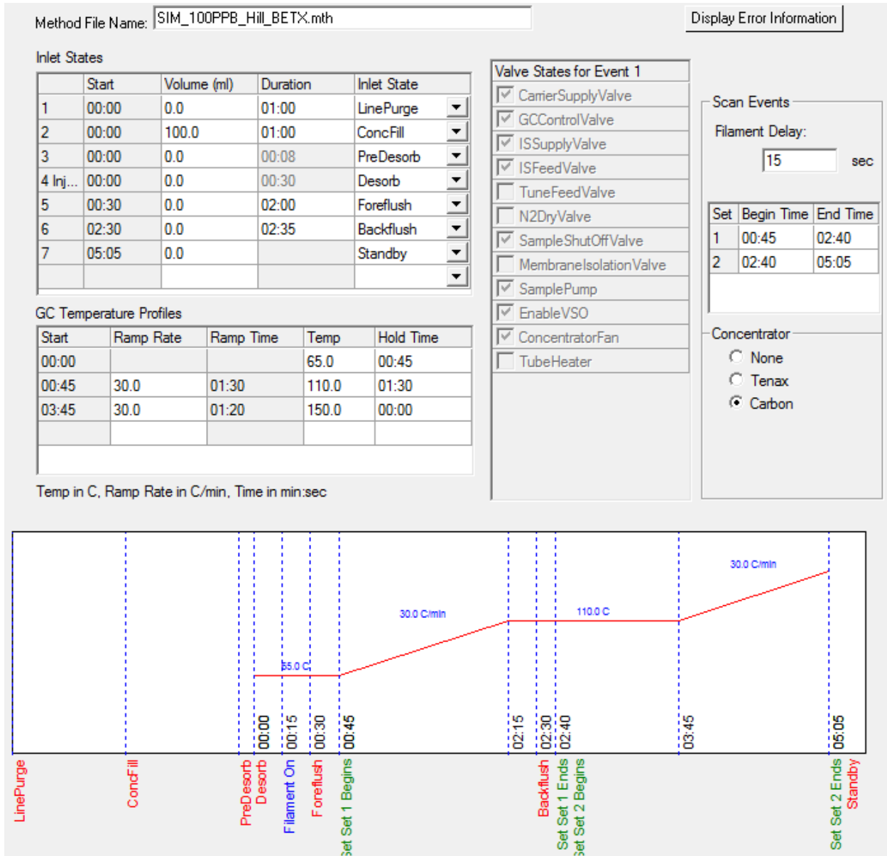
Figure 10: Volume/duration of inlet states, GC temperature profile, and timing of SIM sets in the Petroleum VOCs Method
