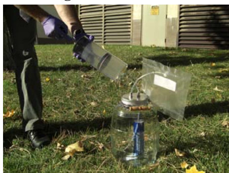
Figure 18: Testing a Potential Indoor VOC Source
