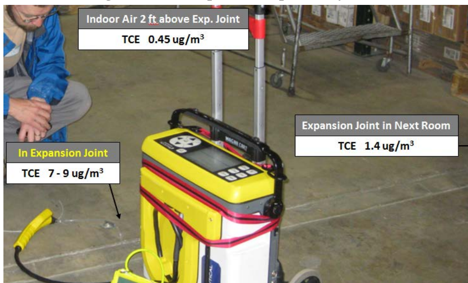
Figure 10: Example of a Vapor Entry Point
