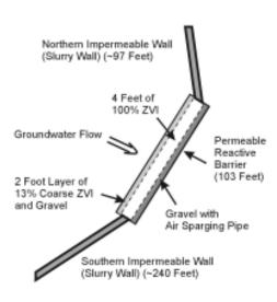
Schematic of PRB at Monticello
