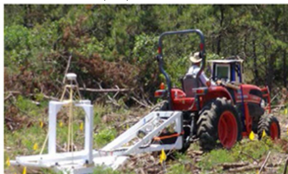
Figure 1. Deployment of MetalMapper at Camp Edwards through a sled configuration.
