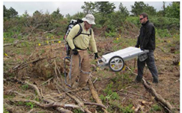
Figure 2. TEMTADS deployment at Camp Edwards involving a backpack-mounted data acquisition computer; a second operator controlled data collection through use of a personal data assistant communicating wirelessly with the data acquisition.
