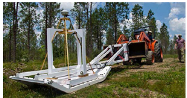
Figure 2. MetalMapper deployed onsite for data collection in cued mode.
