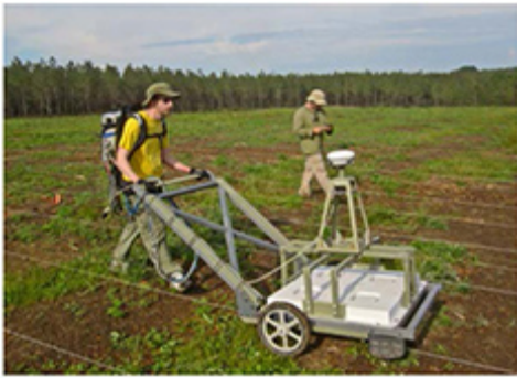
Figure 3. Deployment of TEMTADS 2x2 along closely-spaced parallel transects in the dynamic area at the former Spencer Artillery Range.
