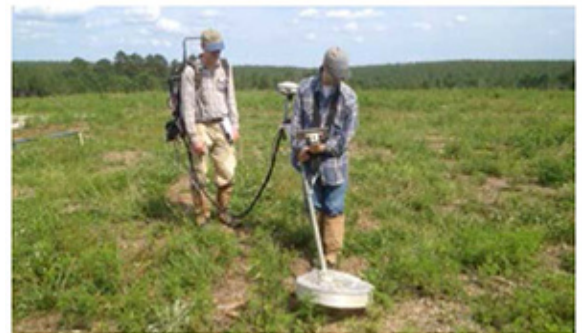
Figure 4. The MPV sensor was deployed in both treed and dynamic areas in cued and dynamic modes at the former Spencer Artillery Range.
