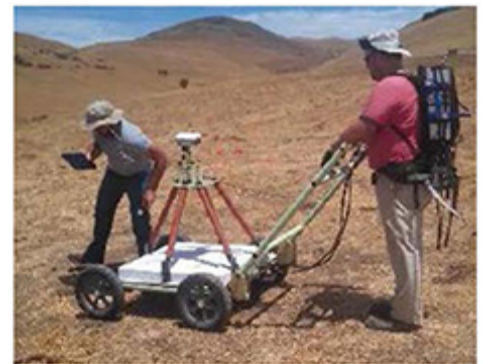
Figure 3. Onsite use of the TEMTADS 2x2 on transects assuming an 0.8-meter footprint.
