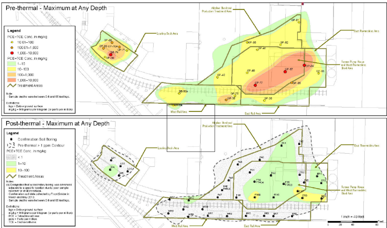
Figure 6. Site-wide reduction in PCE + TCE concentrations due to ERH application.
