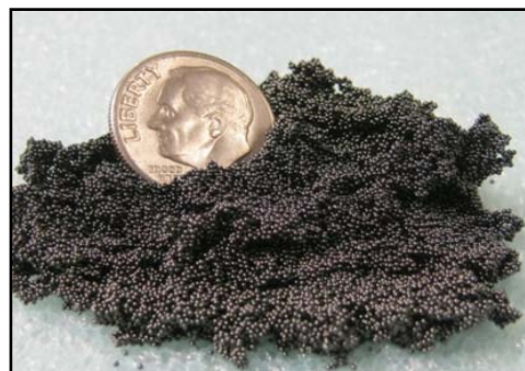
Figure 1. Carbonaceous adsorbent, with non-dusting spherical form.
