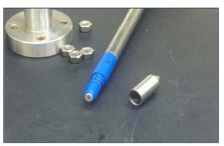
Figure 1. Acoustic probe tip and microphone embedded in the Delrin isolator.
