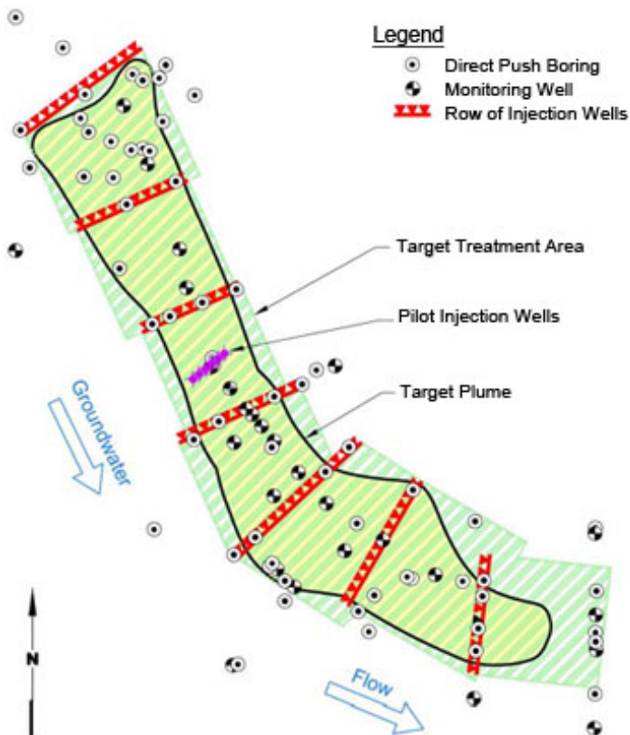
Figure 1. Feasibility study area with seven rows of wells to inject electron donor substrate and bacterial inoculum.
