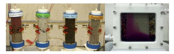
Figure 2.8. 1-D Column Tests (left), and RemOx SR Mini-cylinder 2-D Tank Experiments (right).
