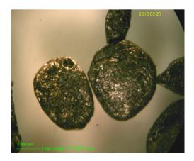
Figure 2.4 Photograph of Slow-Release Permanganate-Wax Pastilles
