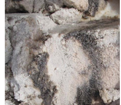
DNAPL at 70 ft bgs
