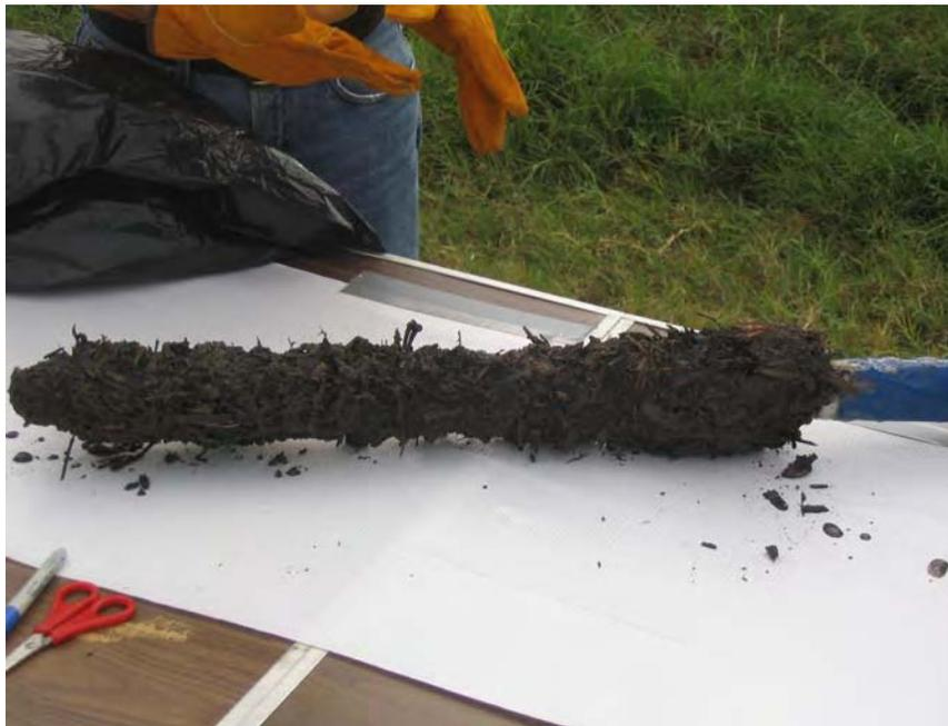
**Figure 6.2 Frozen Sample of Biowall Material Collected Using Liquid Nitrogen Method at Altus AFB, Oklahoma**
