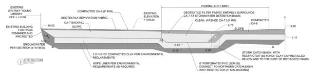
**Clay Barrier Design:** The engineered barrier consists of a geotextile bottom liner, a 3-foot layer of compacted clay and a top layer of gravel mixed with sand.
