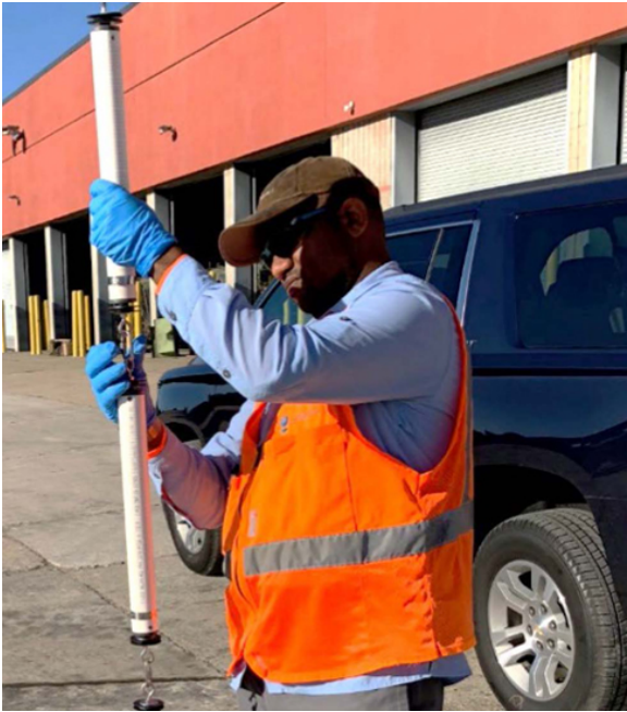
Passive Groundwater Sampling: Bio-Trap ® samplers were deployed in Site 73 monitoring wells to help understand the biodegradation potential and determine the ERD/bioaugmentation approach.
