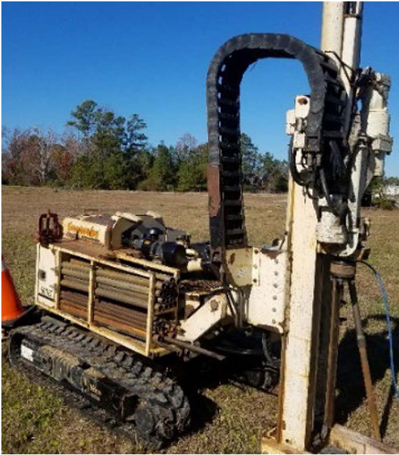
MIP Deployment: A MIP was advanced into targeted subsurface areas via direct push rigging to characterize the subsurface contaminants and identify source areas. The MIP measured volatile hydrocarbon and solvent contamination as well as soil electrical conductance and permeability at various depths in real time.
