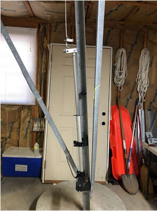
Brake Arm Attachment: A single cable attaches the automatic brake arm to the windmill tail.
