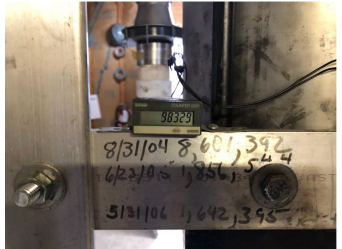
Windmill Stroke Counter: An automatic stroke counter is attached to the cylinder of the windmill stroke arm; every oscillation of the arm is one stroke. The number of strokes over a given time is used to estimate the rate of soil vapor extraction.
