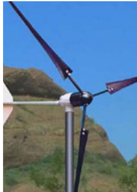
Wind Electric Generator: Four Whisper 200 mast-mounted wind electric generators provided electrical power for submersible pumps prior to 2011. Each generator provided 6.8 kWh per day in a 12 mile per hour average wind.
