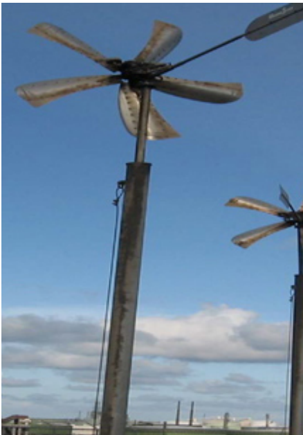
Wind Power Assembly: Prior to 2011, each turbine compressor was powered by a windmill that began rotating at a wind speed of 4 mph. When wind speed exceeded 30 mph, the blades furled and turned out of the wind. The air compressor was located behind the blades at the top of the tower, which was hinged to allow lowering of the full assembly for maintenance or protection from storms. Capital costs for the four units totaled approximately $20,000.
