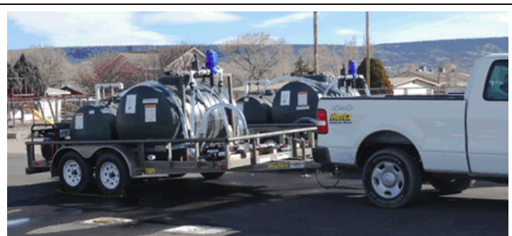
Figure 5. Emulsified Oil Injection Trailer.
