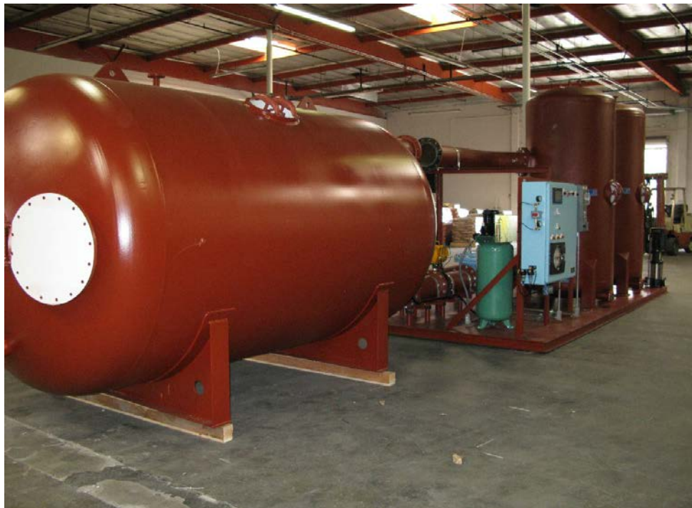
Figure 3-1F. 550-gpm Electromedia® I Filtration System by Filtronics
