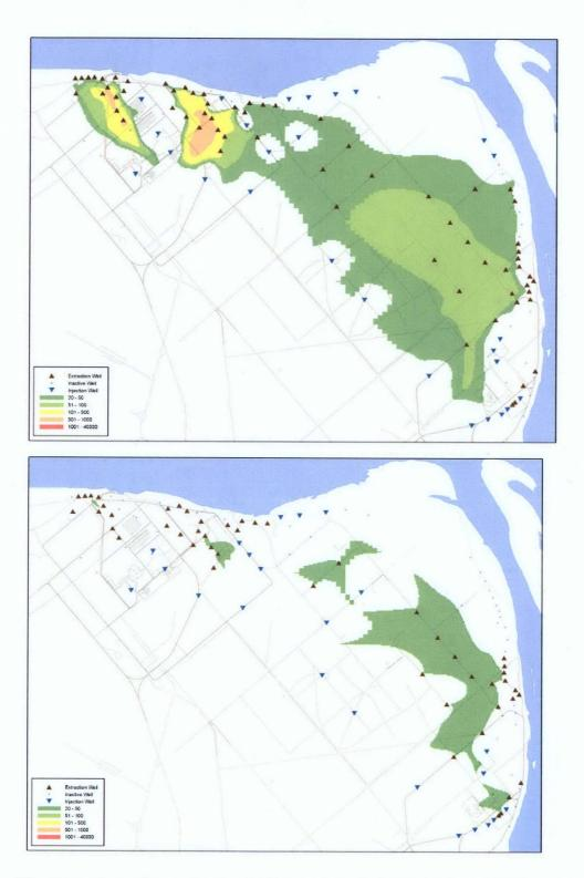
Fig. 4. Projected Remediation in Groundwater, 2012 (top) and 2020 at the 100-HR-3 OU
