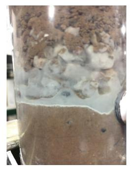
Figure F.10: Injection port on QAL column Day 16 shows the white scale formation at the injection port
