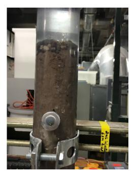
Figure F.8: Injection port on UMCf column Day 16
