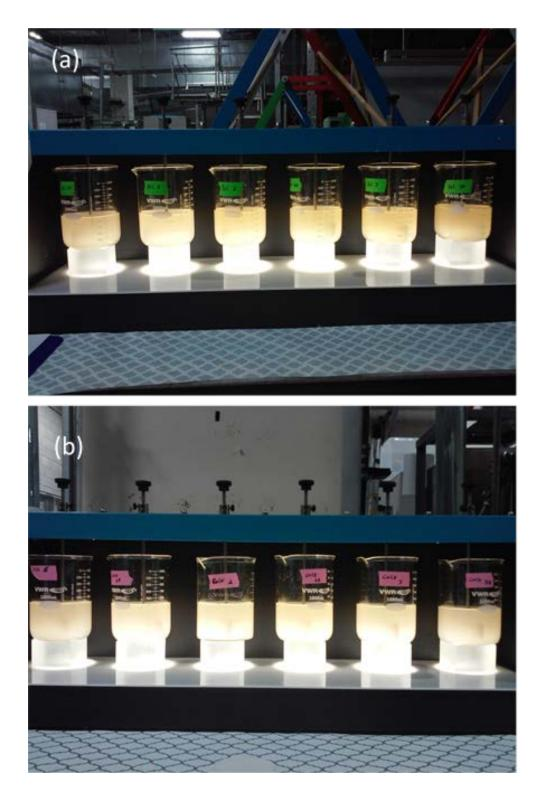
Figure F.3: Low-range concentration batch experimental set-up for QAL groundwater (25 -30 feet bgs) (a) groundwater with ferrous sulfate and (b) with calcium polysulfide.
