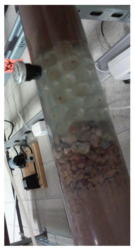
Figure F.12: Injection port showing with gravel and glass beads.
