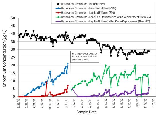
Figure 4-6. WBA Breakthrough Curves for Cr(VI) by Date
