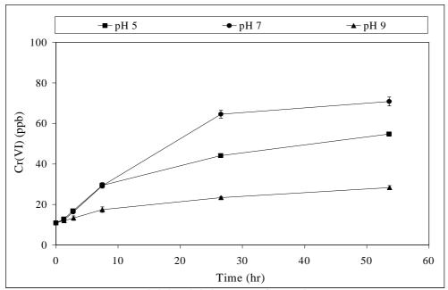
Figure 3-3. Reoxidation of Cr(III) to Cr(VI) with 1 mg/L Free Chlorine in Glendale Water
