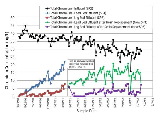
Figure 4-8. WBA Breakthrough Curves for Total Cr by Date
