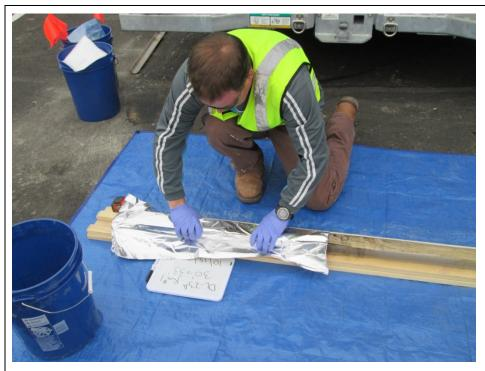
**Step 3.** After the core was photographed it was quickly covered with foil in order to minimize volatile losses.
