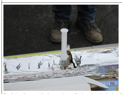
**Step 4.** A marker was used to demarcate the sampling intervals on the aluminum foil. When it was time to sample a particular interval, the foil was pulled back. Four subsamples were collected at each depth interval for laboratory analysis of VOCs, Oil-Red-O dye shake tests, DyeLIF screening, and moisture content.
