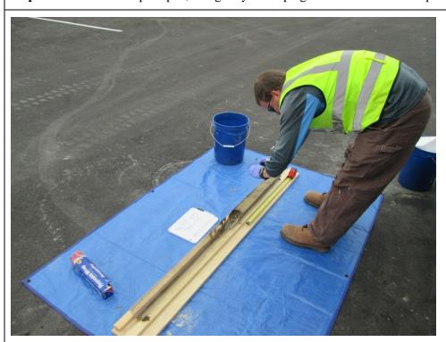
**Step 2.** A photograph of the core was taken. The dry-erase board shown indicates the location ID and core run
