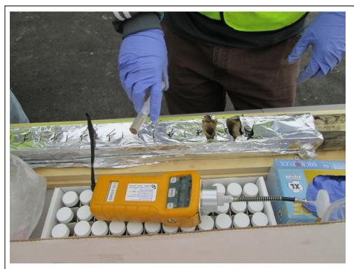
**Step 6.** After sampling is completed at one depth interval, foil from the next interval is pealed back and the process is repeated.
