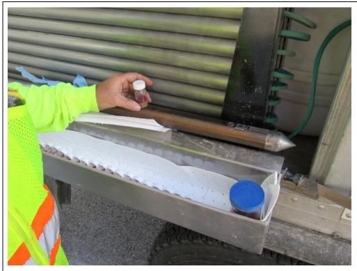
This photograph depicts the procedure used for the aboveground DyeLIF testing. A small amount of dye solution is added to the sample vial and the vial is placed on the probe laser/window and slowly rotated while reading are collected.
