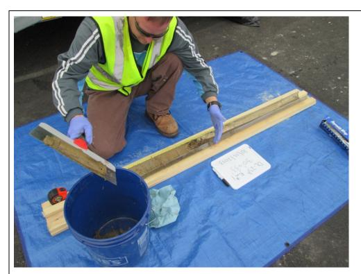
Step 1. After the ore is split open, a large drywall taping knife was used to scrape off the top layer of soil.
