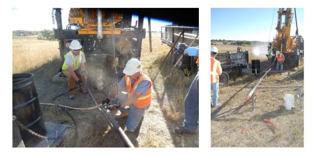
Figure 3-24. Application of hot water to the cooling coils to release the sample liner
