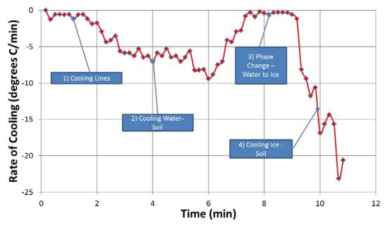
Figure 3-26. Observed rates of change of temperature within the core liner
