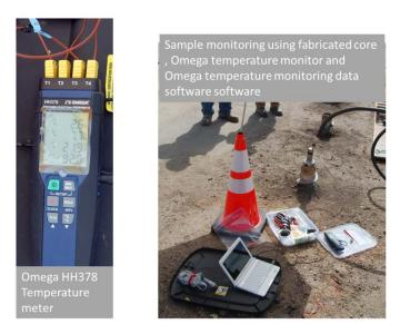
Figure 3-14. Temperature monitoring equipment for fabricated core
