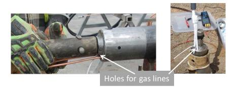
Figure 3-6. Modifications to the CME continuous sample tube system
