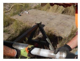
w. Cut the core as desired, cap both ends, and label the core.
