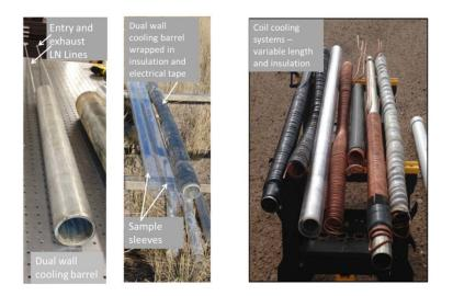
Figure 3-9. Dual-wall cooling cylinder, insulated cooling cylinder, and coil cooling system
