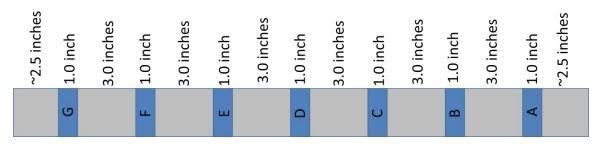
Figure 4-4. Typical Sampling Pattern for Frozen Cores
