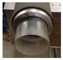
e. Screw the drive shoe onto the core barrel
