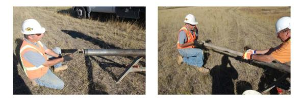
Figure 3-23. Extraction of Sample Liner
