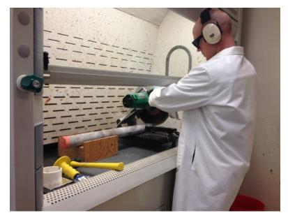
Figure 4-3. Photograph of frozen-core cutting
