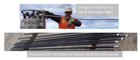
Figure 3-11. Liquid nitrogen supply and exhaust lines
