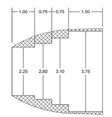
Figure 3-7. Dimensioned drawing of modified drive shoe
