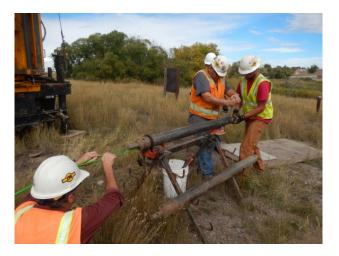
d. Insert the core liner into the core barrel.
