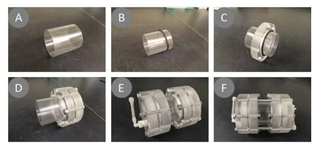
Figure 4-8. Assembly of core-in-liner K-testing apparatus: (A) An empty core-sampling liner, (B) liner with one O-ring in place, (C) with collar, (D) with collar/end-cap assembly, loosely bolted with short bolts, (E) with second collar/end-cap assembly in place, and (F) with long-bolts in place
