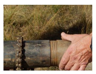
f. Connect core barrel to hex rod
