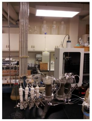
Figure 4-9. Falling head test station
