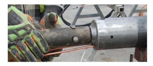
g. Connect LN riser tubes to the cooling coil tubes
