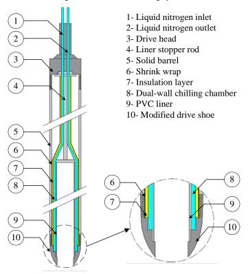
Figure 3-20. Dual-Wall cooling cylinder system design
