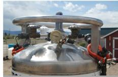
Supply tank pressure control valves, pressure gauge, and level gauge
