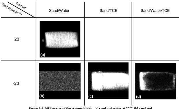
Figure 5-4. MRI images of the scanned cores. (a) sand and water at 20°C, (b) sand and water at -20°C, (c) sand and TCE (100% pore saturation) at -20°C, and (d) sand, water, and TCE (variable pore saturation) at -20°C
