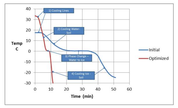
Figure 3-25. Temperature versus time data for freezing samples
