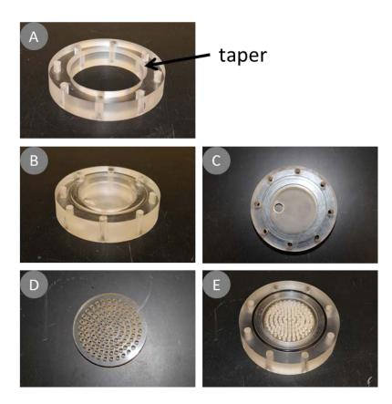
Figure 4-7. Components of core-in-liner K-testing apparatus: (A) collar, (B) end cap, (C) end cap overhead view, (D) filter disc, and (C) end cap overhead view with filter disc emplaced
