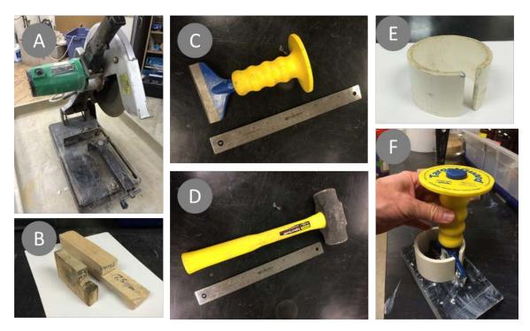
Figure 4-1. Materials and equipment used for high-throughput core processing. The following are shown: (A) cut-off saw, (B) stop blocks, (C) chisel, (D) hammer, (E) PVC pipe, cut to size, and (F) entire apparatus used for sub-dividing frozen core discs.
