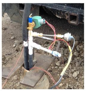
t. During core extraction to ground surface the LN riser tubes and the hex rod must be sequentially removed. (Note: depending on the depth, 20-foot sections of the hex rod and riser tubes may be taken off at a time to speed the process.)
