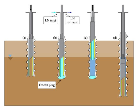
Figure 3-22. Drilling and sampling sequence
