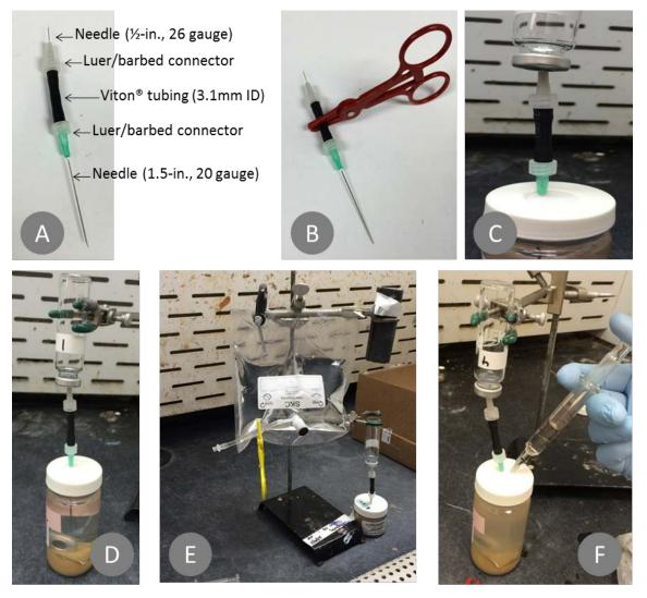
Figure 4-6. Photographs of the aqueous-extraction transfer procedure. Aqueous transfer device shown (A) with parts labeled, (B) with clamp, (C) connected to headspace vial and aqueous-extract jar, (D) aqueous extraction vial/headspace vial assembly, with the headspace vial supported by a ring-stand clamp, (E) Tedlar bag, and (F) injection of water to complete the transfer of aqueous extract into the headspace vial
