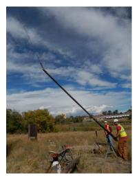
u. Loosen and remove the drive shoe
