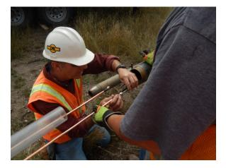
c. Pull/push the cooling coil/cylinder into core barrel
