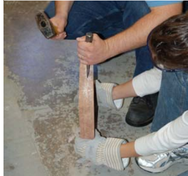
Figure 3-3. Inducing fractures. Fractures were induced along natural mineral bedding planes of the sandstone rocks.
