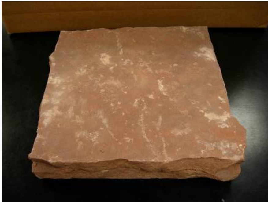
Figure 3-2. Top face of Colorado sandstone. Rock dimensions are 29 cm x 29 cm x 5 cm.
