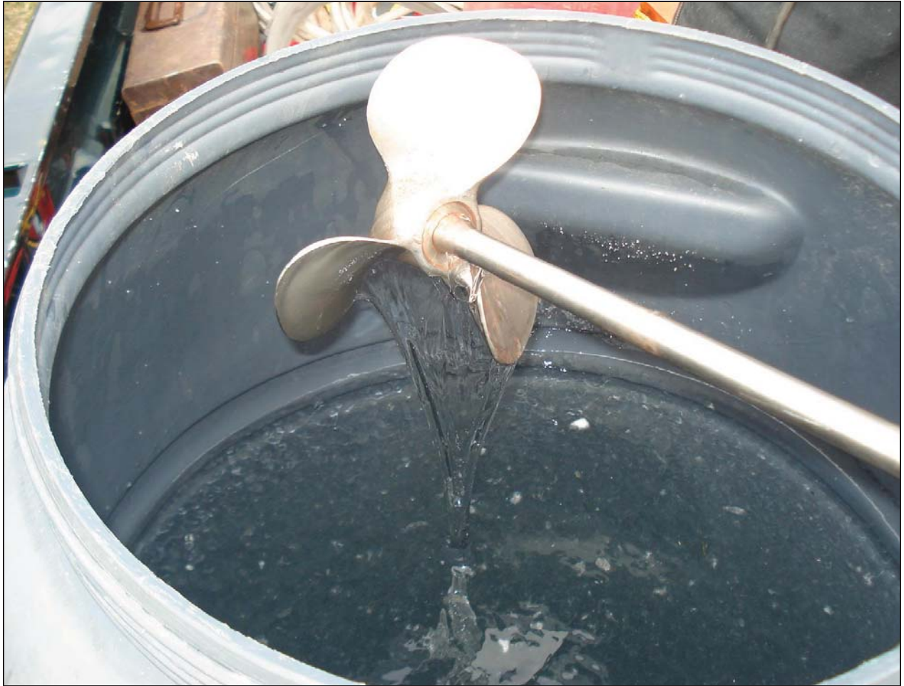
Figure 5-17. Stock solution of SlurryPro™ (0.2 wt%).
