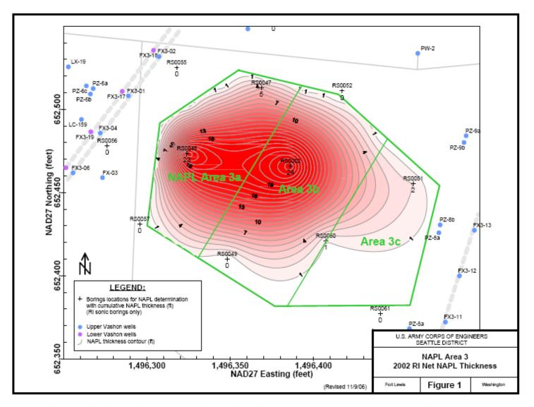
Figure 2. Inference of NAPL distribution within NAPL Area 3 based on data gathered during the Phase 2 RI (2002) (USACE, 2008). Boxes highlighted in blue indicate target treatment cell locations.
