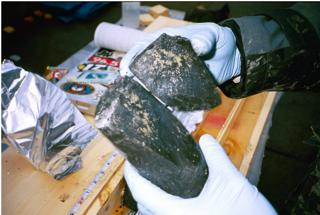
Figure D-4: Example photos of field core samples with pyrite accumulation on fracture surfaces.
