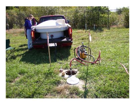
Figure 4. Reagent Mixing and Injection System Photograph—HAFB.
