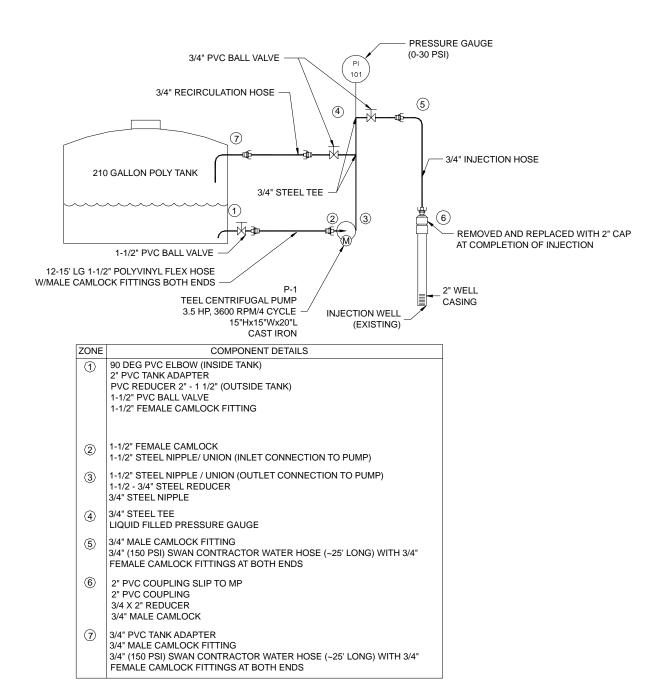
Figure 3. Reagent Mixing and Injection System Schematic—Vandenberg Air Force Base (VAFB).
