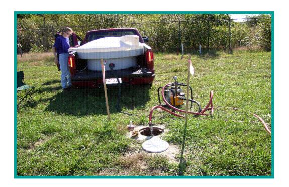
In-situ Substrate Addition to Create Reactive Zones for Treatment of Chlorinated Aliphatic Hydrocarbons
