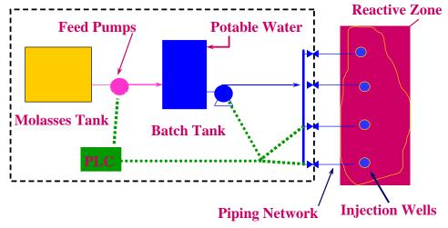
Figure 2. Conceptual Design for an ERD System Layout.
