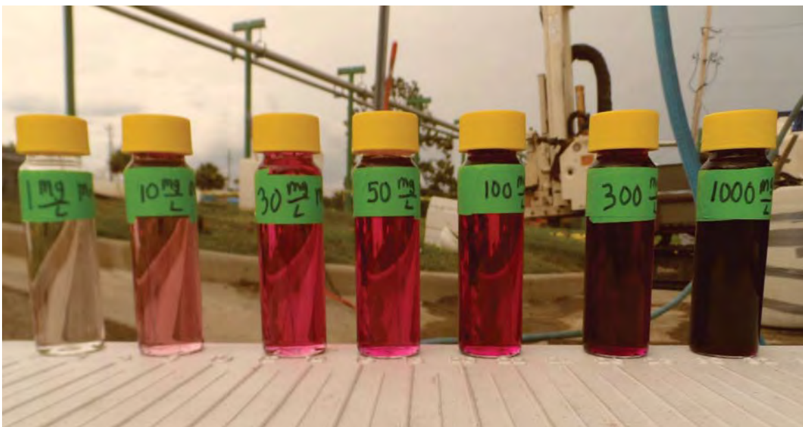
Photo 36. The color of the sodium permanganate solutions at different concentrations were prepared to provide a field “quick test” to approximate permanganate concentrations.
