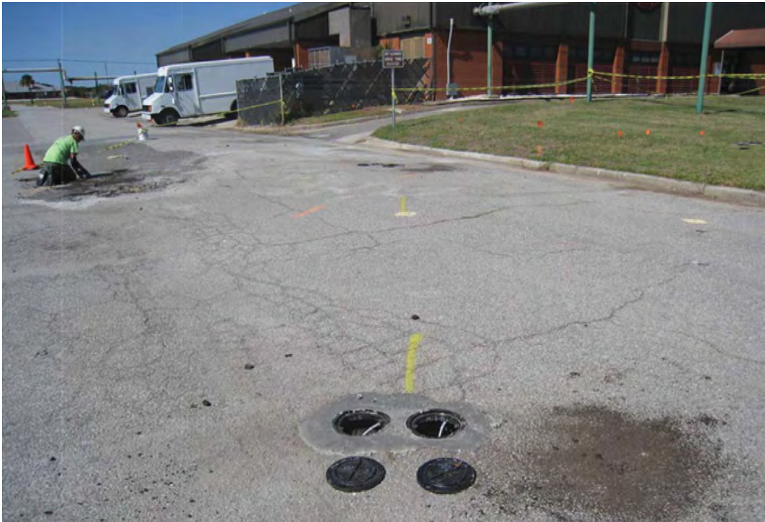
Photo 15. Looking upgradient from the middle of Kyushu Street towards the new Dry Cleaner building. The approximate centerline of the plume (yellow) is from the corner of the dry cleaner building and extends in the southeastern direction. The open, flush-mounted micro-wells (M3-mid-shallow and M3-mid-deep) are shown in the immediate foreground.
