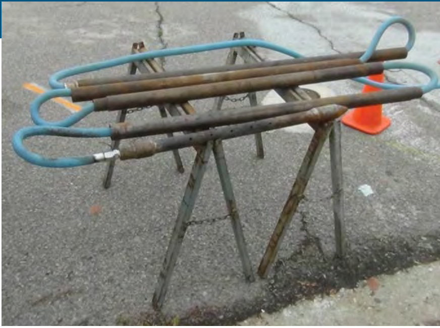
Photo 20. The oxidant injection line is strung through each of the GeoProbe rods needed to achieve the target depth at each location. The direct push injection tip, GeoProbe rod, and injection hose connected prior to injection.
