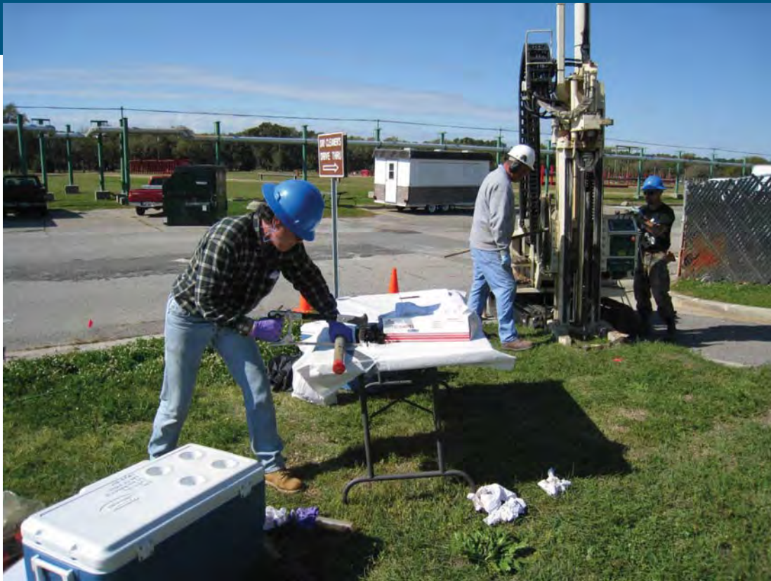
Photo 7. Soil core collection using a GeoProbe (background), and soil core processing (capping, cutting, sealing, and freezing) for shipment to RSKERC facility for analysis.
