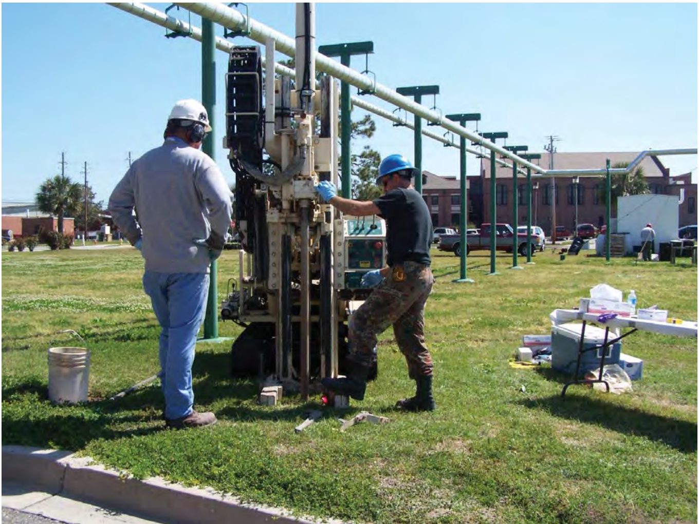
Photo 6. Retrieving soil cores using the GeoProbe equipment along transects extending across (perpendicular) the ground water plume.
