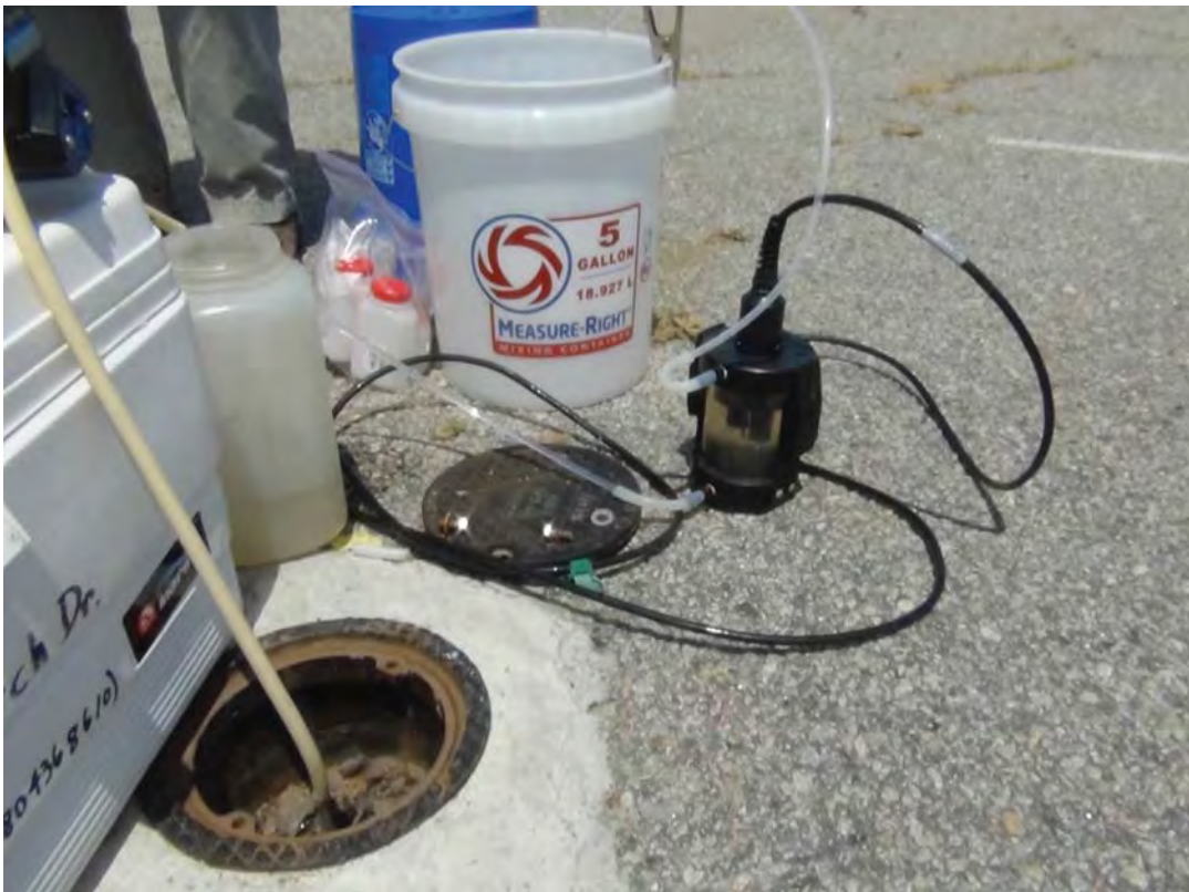
Photos 16-17. Post-installation development of micro-wells was carried out by pumping ground water at a slow rate. A few liters of ground water was generally required to “develop” the micro-wells until stabilized general parameters and clear ground water could be achieved.
