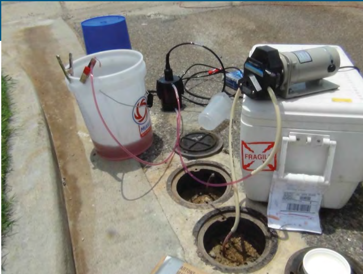
Photo 35. Ground water sampling at micro-wells involved “binary mixtures” of ground water and the oxidant solution that was injected as seen by the pink-purple color in the tubing. Ground water samples exhibiting presence of \text{NaMnO}_4 were neutralized using ascorbic acid.
