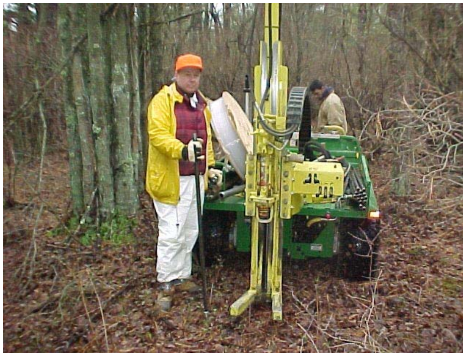
Figure 9. Direct-push GeoProbe rig mounted onto a John Deere Gator. (The narrow width of the Gator allows access to difficult-to-reach locations within swamp-like wetlands.) USGS photo
