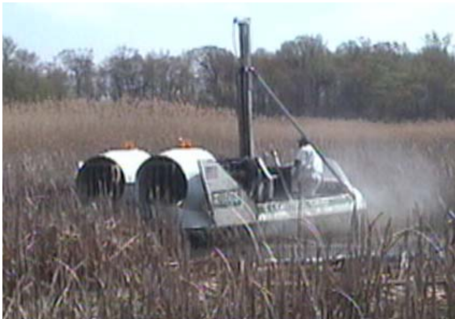
Figure 8. Vibracore systems used at the West Branch Canal Creek wetland site at Aberdeen Proving Ground, MD: (upper left) portable hydraulic unit with vibration only; (upper right) portable hydraulic unit with vibration and hammer action; and (lower) hoverprobe with attached hydraulic vibracore unit with vibration only.
