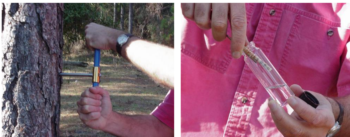
Figure 10. Tree core sampling procedure for analysis of chlorinated volatile organic compounds: (left) tree coring using standard forestry coring device, and (right) addition of core to vial containing methanol for extraction. USGS photos
