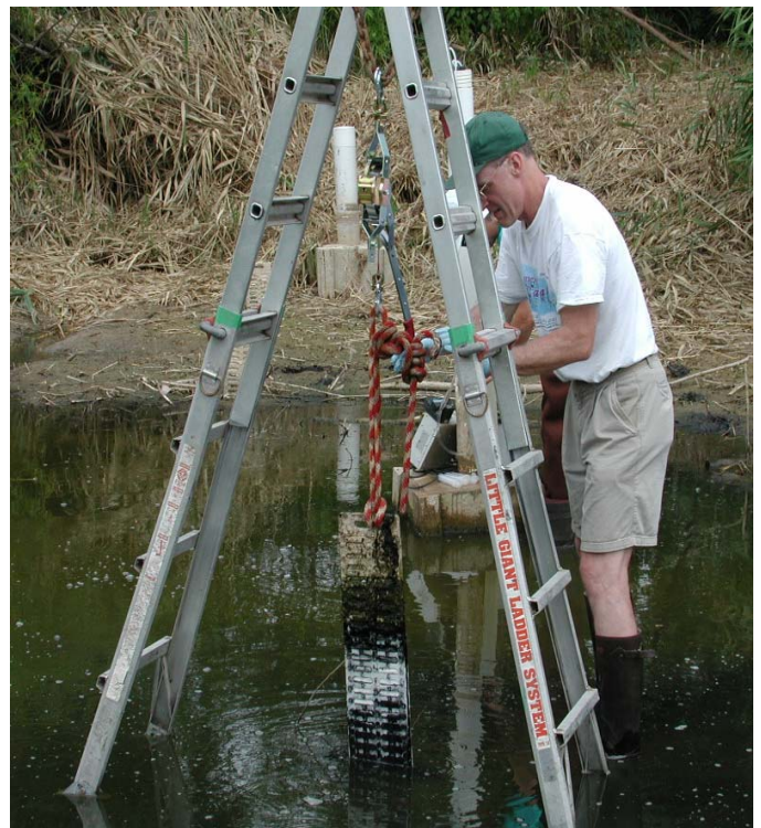
Figure 22. Field recovery and sampling of peepers. (Upper left) Removing peeper from wetland sediment using simple wooden lever system. (Upper right) Withdrawing aqueous samples from peeper chambers for analysis of various parameters to assess natural attenuation of chlorinated solvents discharging into Aberdeen Proving Ground, MD wetland field site. (Lower two photos): Recovering peeper from streambed using a ladder and winch at Norman, Oklahoma wetland site. (The Norman, Oklahoma site is a research site for the U.S. Geological Survey Toxic Substances Hydrology Program.)
