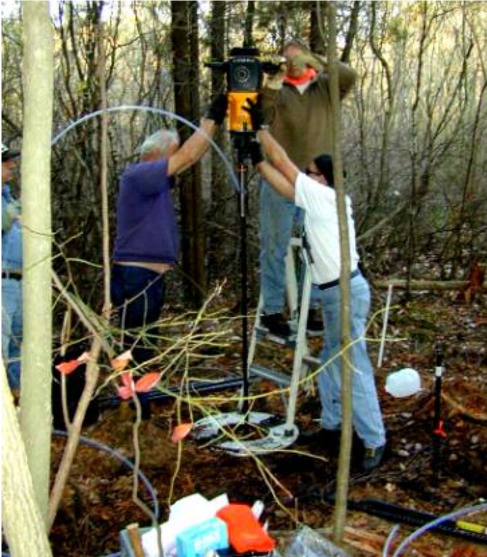
Figure 11. Installation of narrow-diameter drive-point piezometer using percussion hammer. [Note the Teflon tubing inner sleeve extruding out of the hammer adapter. The Teflon tubing is connected by tubing barb to a stainless-steel drive-point tip with screens for ground-water inflow.] (Solinst Canada Ltd. photo)
