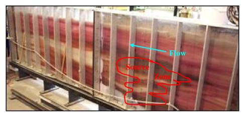
Figure 3.91. Oxidation during ISCO High Heterogeneity Experiment
