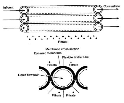
Figure 5-2. Filtrate Polishing using Micro filtration.
