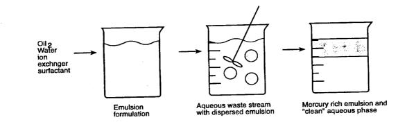
Figure 5-4. Schematic representation of mercury ion extraction with an emulsion liquid membrane.
