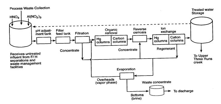
Figure 7-1. F/H effluent treatment facility process flow sheet.
