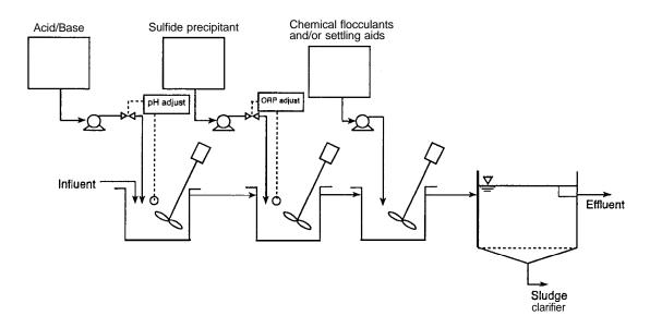
Figure 2-1 Sulfide precipitation.
