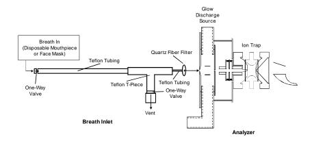
Figure 4-3. Continuous real-time breath analyzer (RTBA), consisting of breath inlet (breath holding volume) attached to direct breath sampling interface (glow discharge ionization source) and ion trap mass spectrometer (GD/ITMS).
