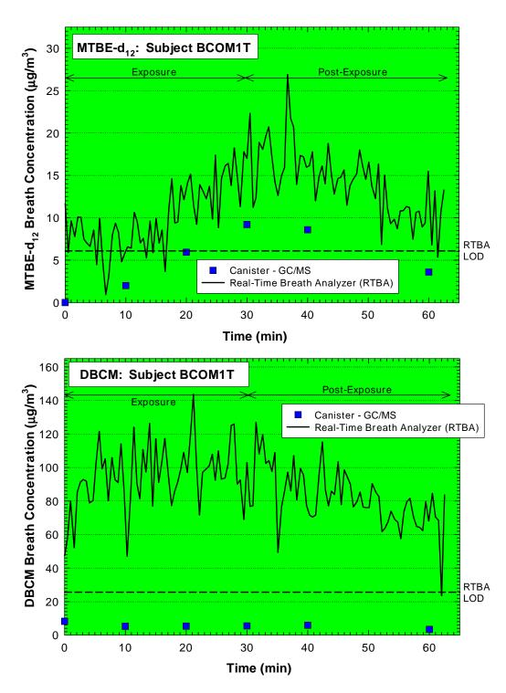
Figure 5-4. Continuous exhaled breath concentrations for MTBE-d<sub>12</sub> (upper plot) and DBCM (lower plot) as a function of time for Subject BCOM1T during and following dermal exposure while bathing. Exposure duration was 34.1 min; post-exposure monitoring continued for another 31.0 min. Water temperature was 39.7°C. Nominal concentrations were 150  $\mu$ g/L for MTBE-d<sub>12</sub> and 40  $\mu$ g/L for DBCM. RTBA LOD designates detection limit with real-time breath analyzer.
