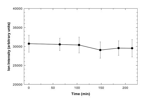
Figure 5-19. Plot of average ion signal (and standard deviation) at m/z 55 as a function of time, obtained from constant source of 2-butanone in glass chamber at a concentration of 866  $\mu$ g/m³ in zero-grade air.
