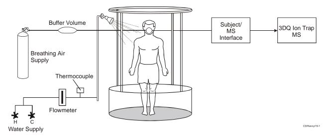
Figure 4-1. System for sampling exhaled breath samples in real time from subject exposed by dermal absorption to MTBE and DBCM in shower water. (Schematic shows only one shower unit for clarity.)
