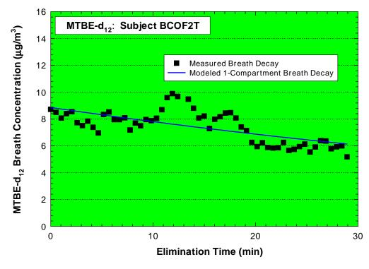
Figure 5-16. Measured MTBE-d<sub>12</sub> exhaled air exposure decay plot for Subject BCOF2T compared with modeled curve. Bath exposure details as described in Figure 5-7. Data smoothed using 5-point moving average.
