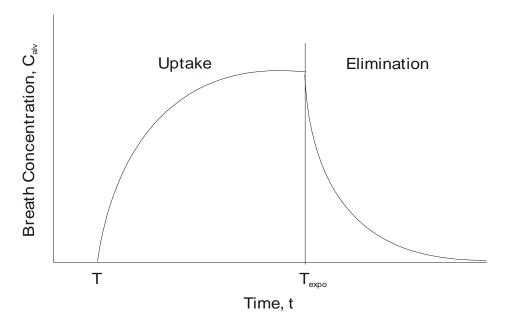
Figure 4-4. Plot showing rapid increase in alveolar breath concentration  $C_{alv}$  as a result of step function exposure to a constant water concentration  $C_{water}$ , followed by a rapid decrease in breath concentration as a result of exposure to clean air. T is the lag time, i.e., the time to the first measurable increase in the breath concentration;  $T_{expo}$  is the time at the end of exposure.
