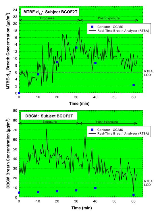
Figure 5-7. Continuous exhaled breath concentrations for MTBE-d<sub>12</sub> (upper plot) and DBCM (lower plot) as a function of time for Subject BCOF2T during and following dermal exposure while bathing. Exposure duration was 33.0 min; post-exposure monitoring continued for another 29.5 min. Water temperature was 39.8°C. Nominal concentrations were 150  $\mu$ g/L for MTBE-d<sub>12</sub> and 40  $\mu$ g/L for DBCM. RTBA LOD designates detection limit with real-time breath analyzer.
