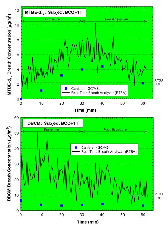
Figure 5-5. Continuous exhaled breath concentrations for MTBE-d<sub>12</sub> (upper plot) and DBCM (lower plot) as a function of time for Subject BCOF1T during and following dermal exposure while bathing. Exposure duration was 33.0 min; post-exposure monitoring continued for another 33.1 min. Water temperature was 39.0°C. Nominal concentrations were 150  $\mu$ g/L for MTBE-d<sub>12</sub> and 40  $\mu$ g/L for DBCM. RTBA LOD designates detection limit with real-time breath analyzer.
