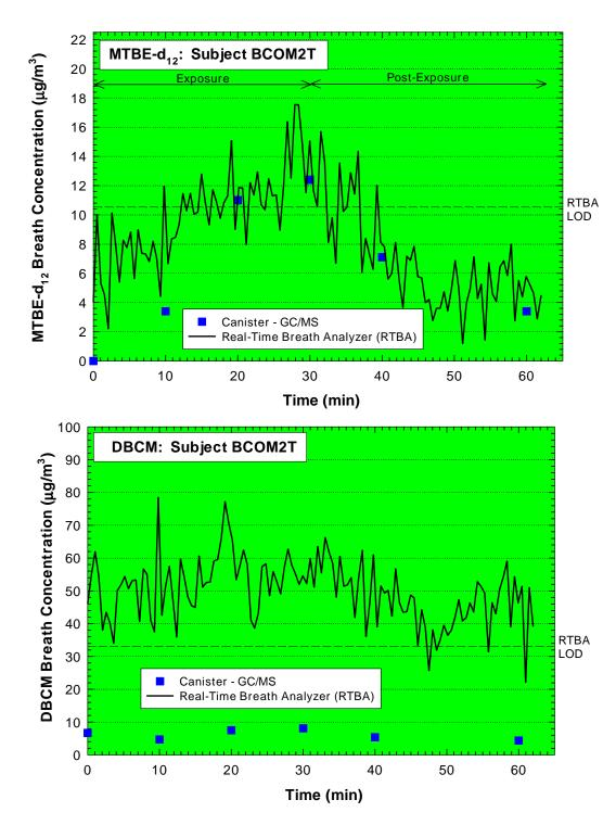
Figure 5-6. Continuous exhaled breath concentrations for MTBE-d<sub>12</sub> (upper plot) and DBCM (lower plot) as a function of time for Subject BCOM2T during and following dermal exposure while bathing. Exposure duration was 33.1 min; post-exposure monitoring continued for another 31.0 min. Water temperature was 38.8°C. Nominal concentrations were 150  $\mu$ g/L for MTBE-d<sub>12</sub> and 40  $\mu$ g/L for DBCM. RTBA LOD designates detection limit with real-time breath analyzer.
