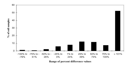
Figure 5-2. Range of percent difference values for the comparisons of the L2000 soil sample results with the reference laboratory results.
