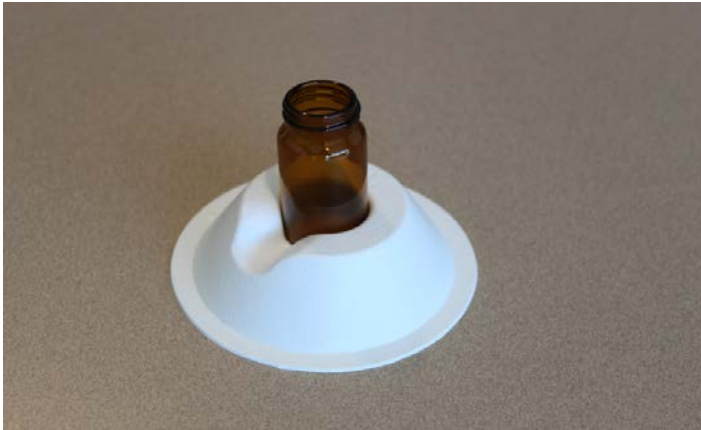
Figure 4.18. Securing the scintillation vial with a centrifuge tube holder
