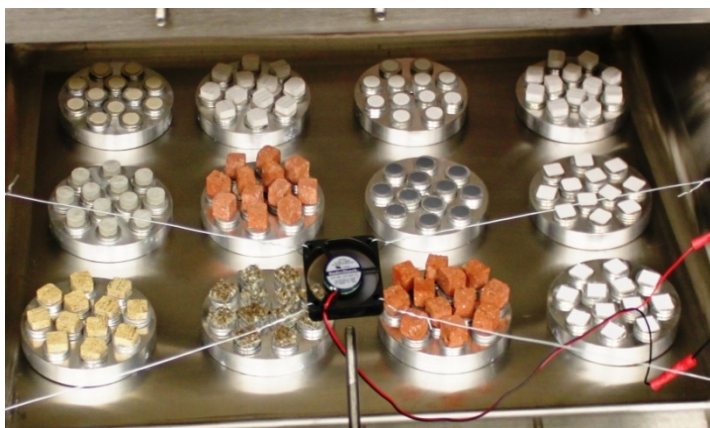
Figure E.2. Sink material buttons that were placed in the test chamber
