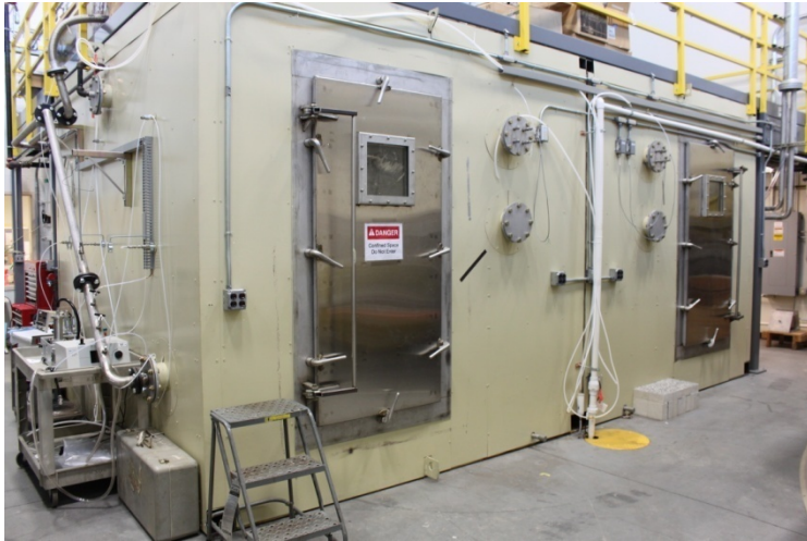
Figure 4.13. Two-Compartment Chamber System (The compartment on the left was used for this study)
