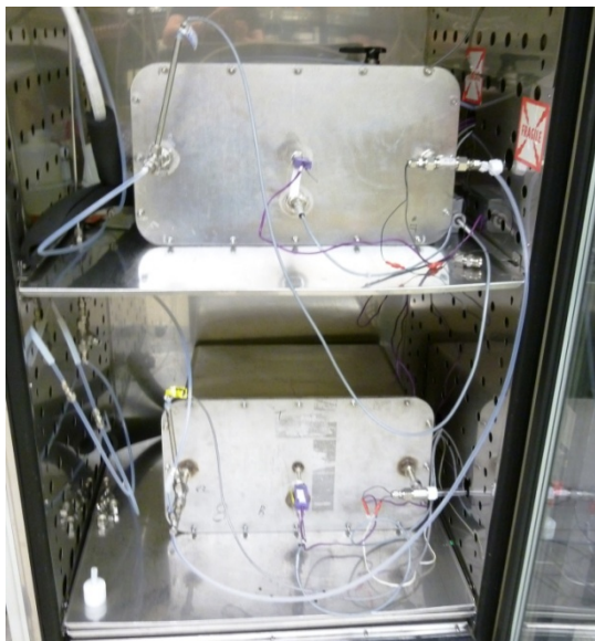
Figure 4.1. Picture of source chamber (top) and test chamber (bottom)
