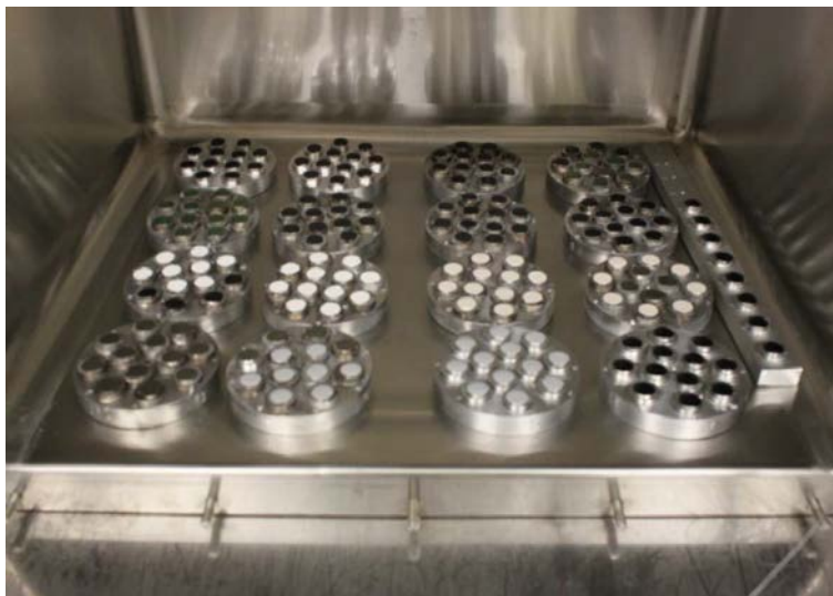
Figure 2.5. Sample stages in the test chamber
