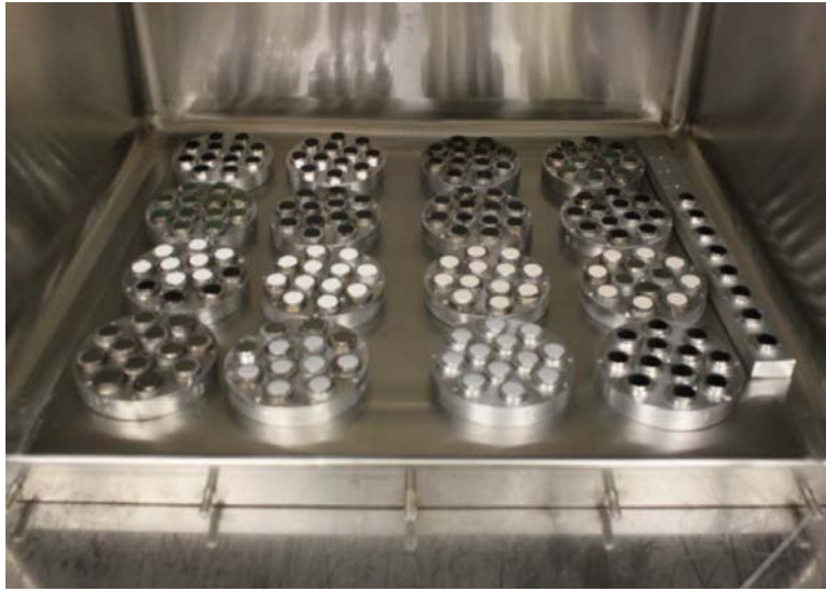
Figure E.2. Encapsulant disks in the test chamber
