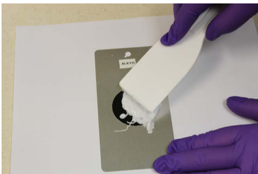
Figure 2.3. Application of inactive AMTS paste to a paint coupon
