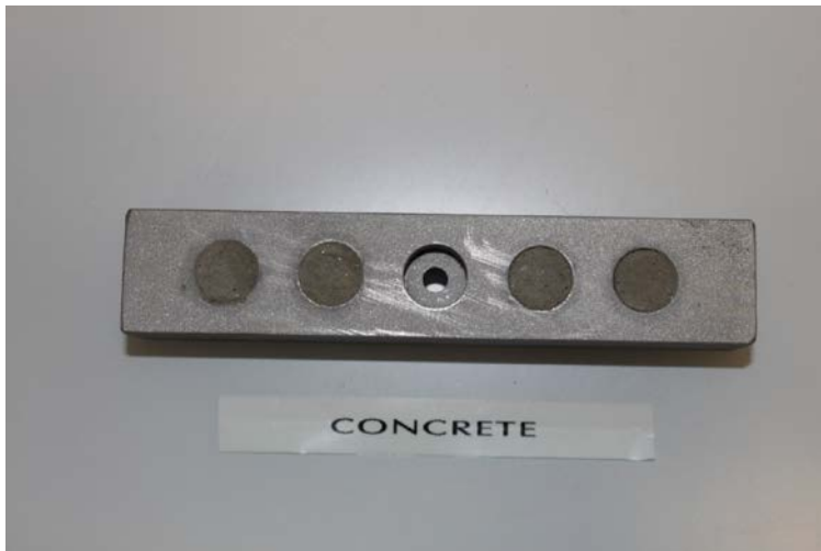
Figure E.4. Concrete pieces in a stainless steel mold for treatment by the AMTS method
