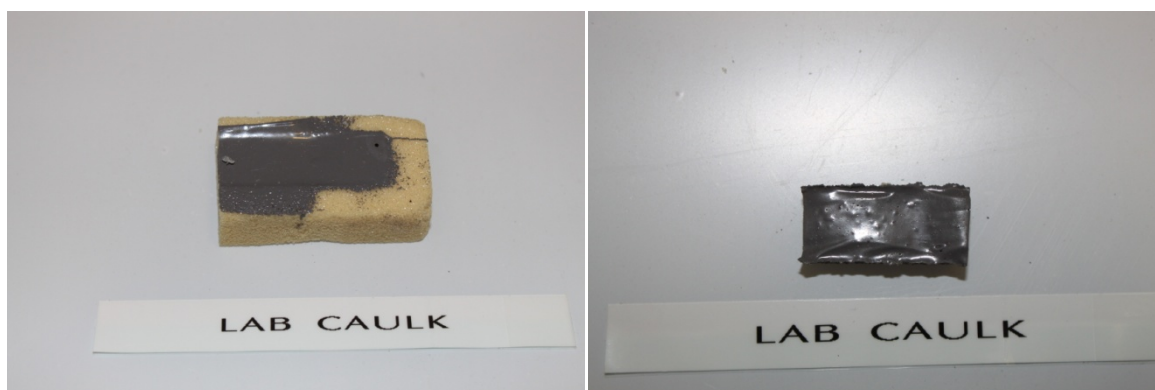
Figure 2.10. Laboratory-made caulk (left: caulk curing in the mold; right: caulk used in tests)
