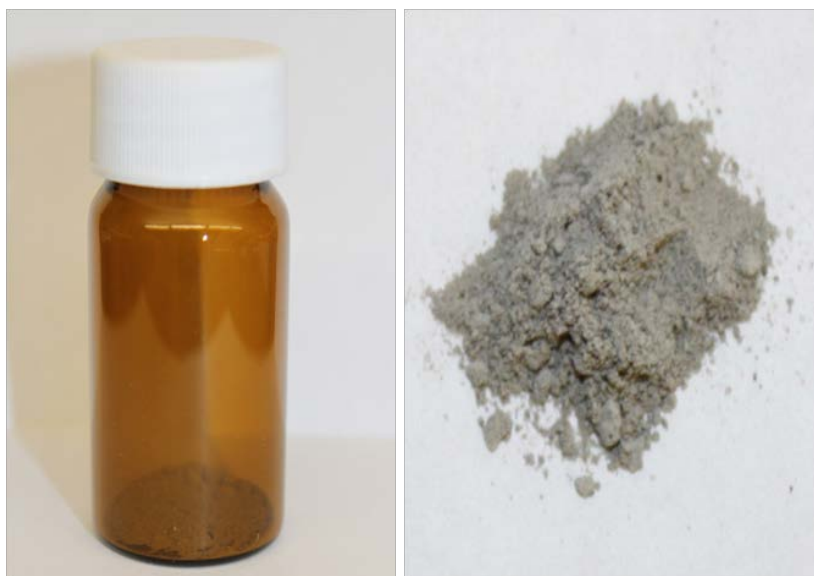
Figure 2.15. Crushed concrete ready for extraction
