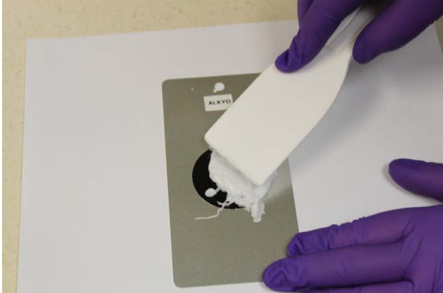
Figure E.2. Application of the inactive paste to a coating coupon
