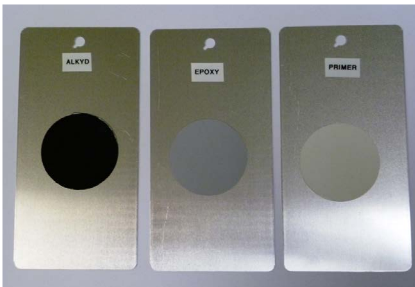
Figure 2.2. Coupons for paint tests (left: alkyd; center- epoxy; right: primer)
