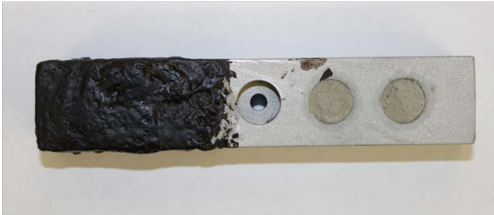
Figure 2.14. Laboratory-made concrete covered with AMTS paste and coating
