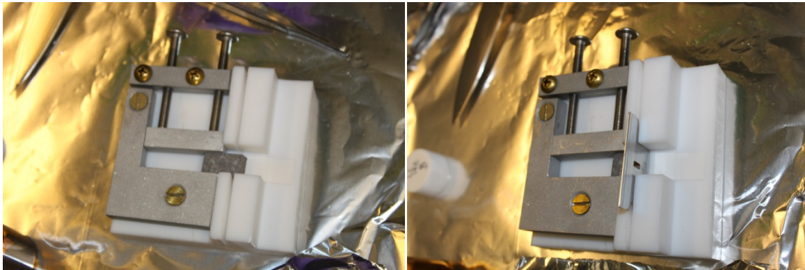
Figure 2.8. Caulk being cut into slices for extraction
