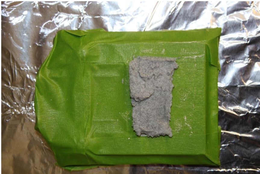
Figure 2.6. Field caulk covered with AMTS active paste
