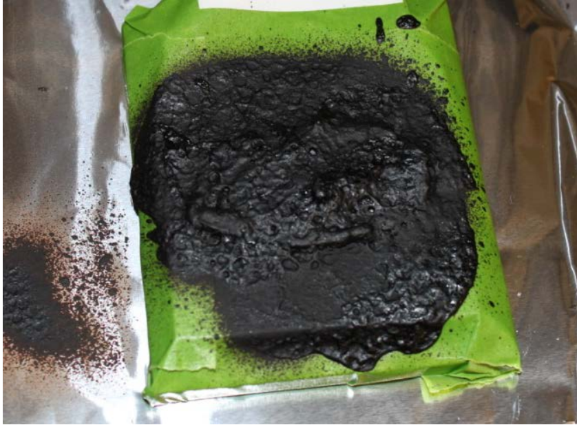
Figure 2.7. AMTS paste covered with the Dupli-Color ® Undercoat
