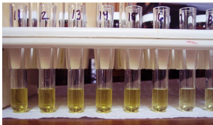
Figure F-3. Typical Immunoassay Run (Note the Subtle Color Difference)
