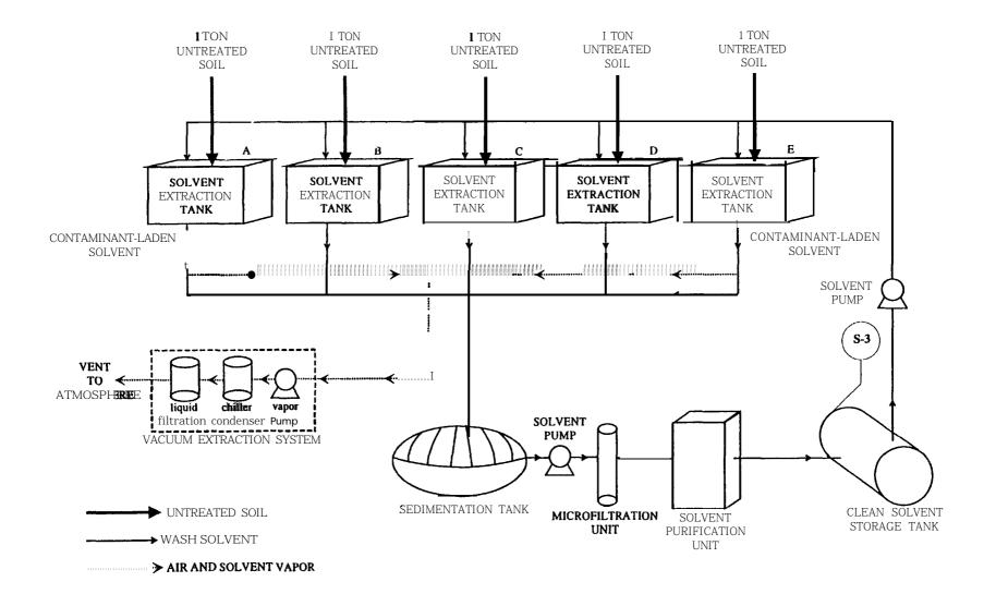
Figure I-I. Schematic diagram of the Terra-Kleen technology.
