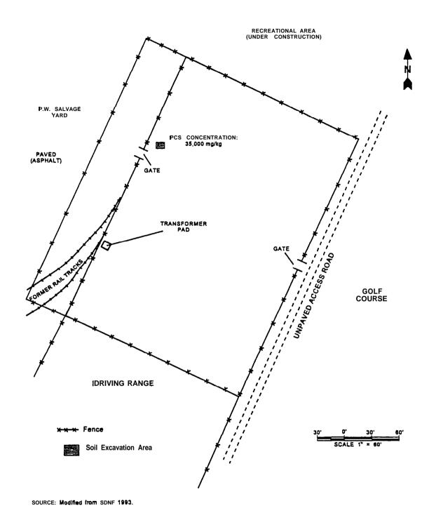
Figure 3-4. NASNI Site 4 PCB contamination and excavation area.
