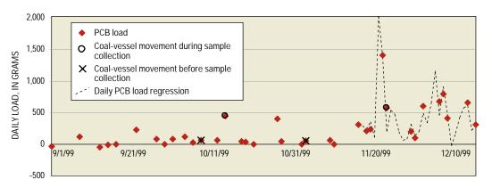
**Figure 9.** Daily water-column PCB load in the deposit area during the dredging operation on the Fox River, Wis.
