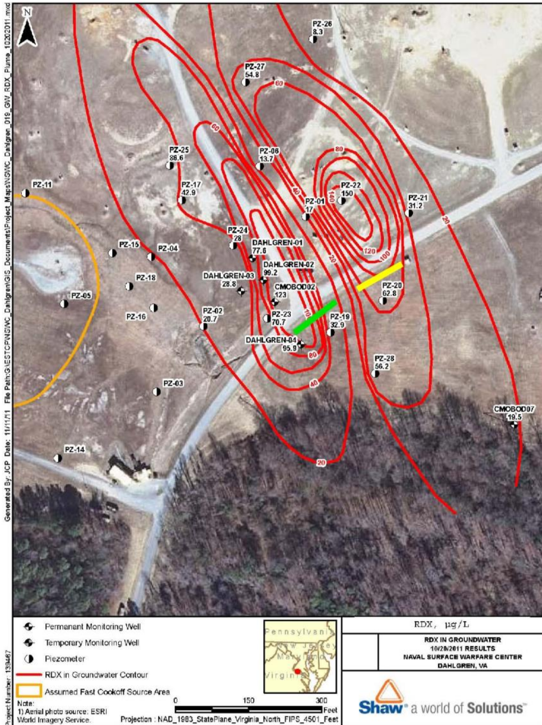
Figure 5.27. Plume map for RDX in the southeast area of the Churchill Range.
