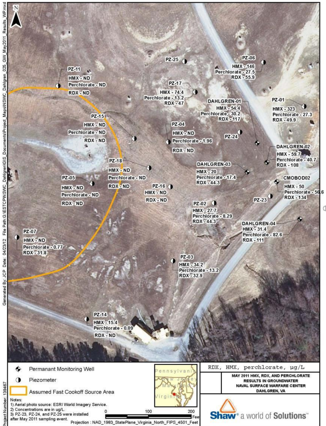
Figure 5.26. RDX, HMX and perchlorate data from piezometers installed during the May 2011 site investigation.
