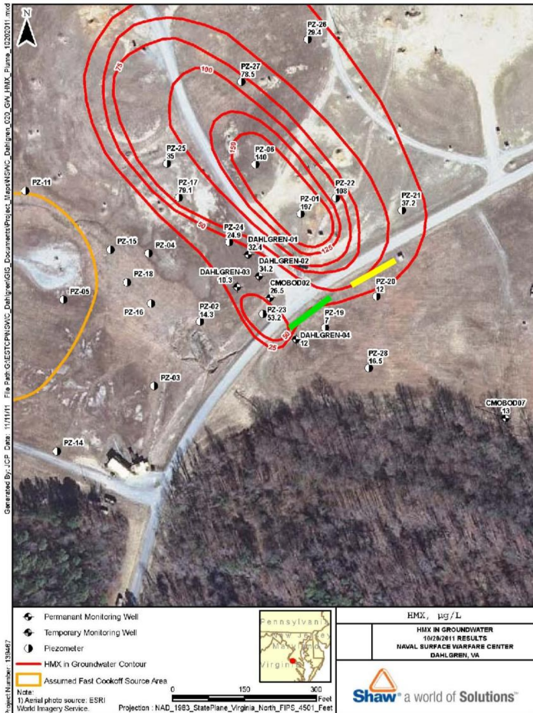
Figure 5.29. Plume map for HMX in the southeast area of the Churchill Range.
