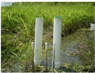
Figure 3-19. In Situ Columns IC-3 and IC-4 adjacent to Piezometer Group 1
