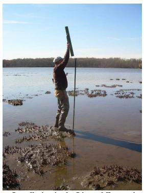
Figure 3-17. Piezometer Installation in the Littoral Zone using a Slide Hammer
