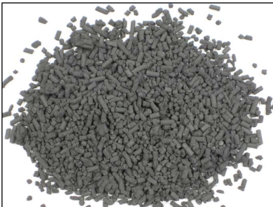
Figure 1. SediMite ® pellets containing powdered activated carbon (PAC). The pellet is an agglomerate that includes the treatment agent (PAC), a weighting agent (sand), and a binding agent. Once wetted, the pellet releases the fine-particle-sized treatment agent to sediments or wetland soils. SediMite ® can include PAC or any other treatment agent or mixture of agents that can benefit from pelletized delivery.
