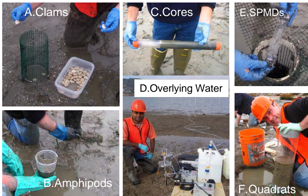
Figure 7. Field samples. (clams, amphipods, sediment cores, overlying water, SPMDs, and quadrats)
